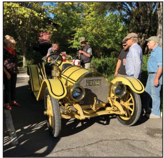
The Mercer 35J Raceabout was arguably one of the world's first supercars. The 300 CID T-head engine made 58 hp and could propel the car to over 90 mph, quite a heady feat for 1913!
