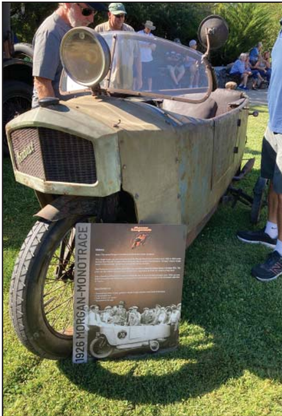
The Morgan Monotrace (which means 'single track') was made by a French company unrelated to the better-known English firm. Licence-built from the German Mauser Einspurauto of 1923, it featured tandem wheels like a motorcycle, with outriggers for 'stability' which folded up when the vehicle was moving. Introduced in 1924, it was powered by a German 510cc single-cylinder engine. Only a handful survived WWII. This one was purchased from the Schlumpf collection in Mulsanne
