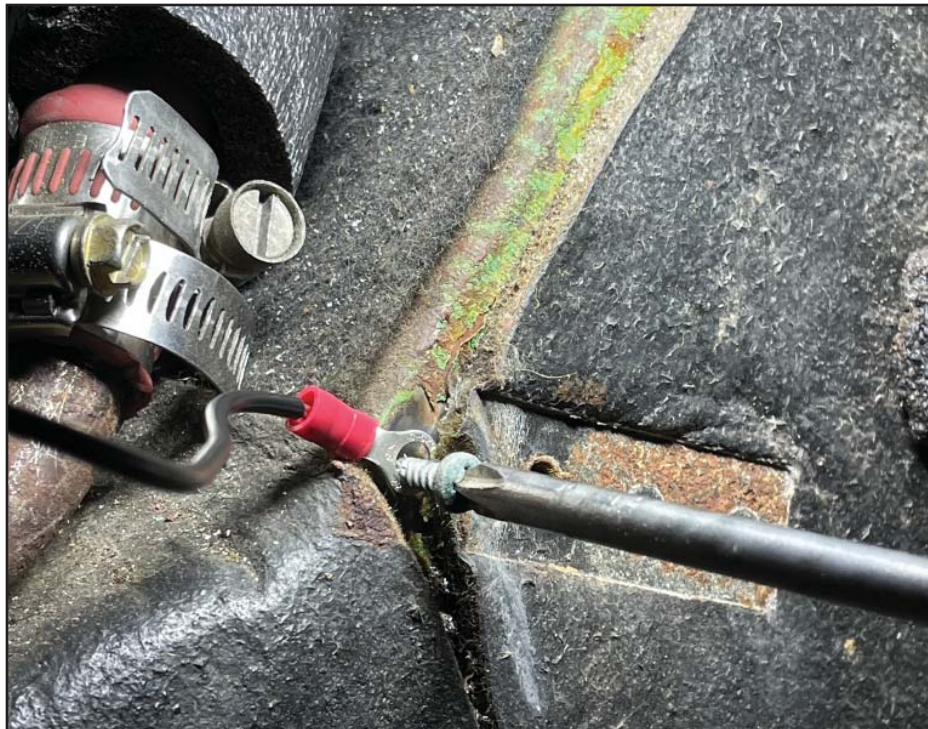
A simple screw and ring connector hidden behind the kick panel proved effective
