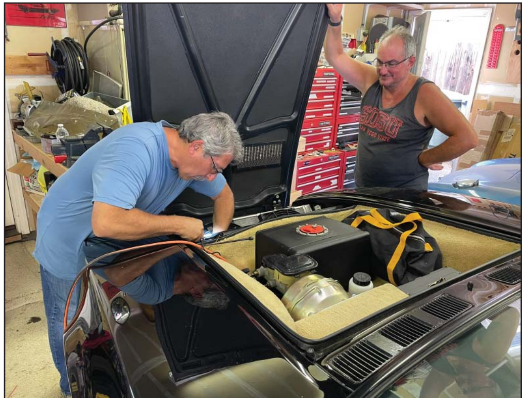
Mark installed the final bolt before crawling underneath the car and pushing up on the mechanism to ensure optimal gear engagement, while I tightened the bolts from above
