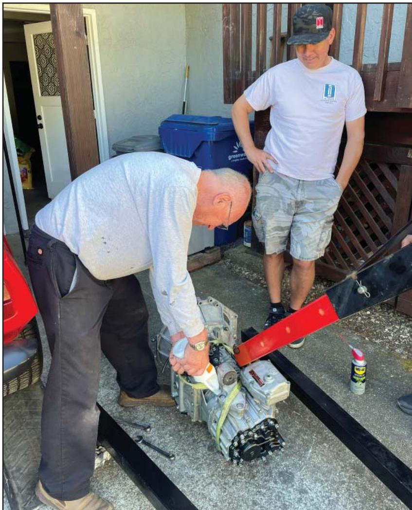
*Forest flipped the gearbox on its side for easy filling with 80W-90 GL-5 lube*
