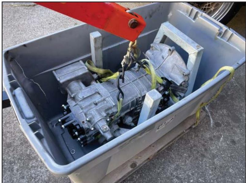
*The gearbox was transported in this custom affair consisting of a welded steel cradle, set inside a plastic tub, and bolted to a wooden pallet*
