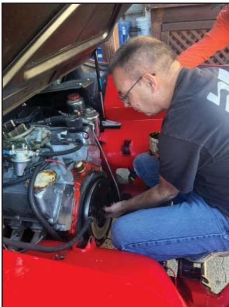
*I thoroughly lubricated the roller pilot bearing with axle grease*
