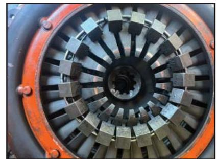
*Despite the lack of a proper clutch alignment tool, Steve managed to get the disc reasonably centered, which was a bit of a miracle*
