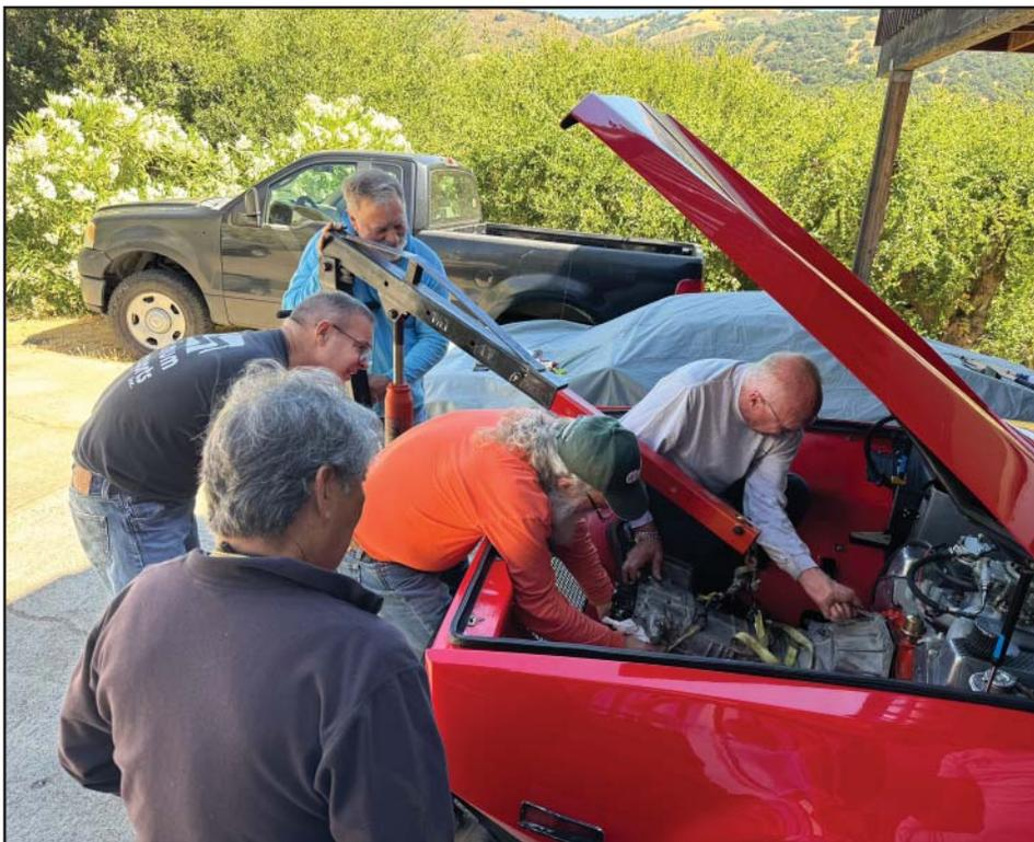
*It proved more than a little bit challenging to get the splines on the input shaft to line up properly with the clutch disc, but eventually the gearbox snicked happily into place*
