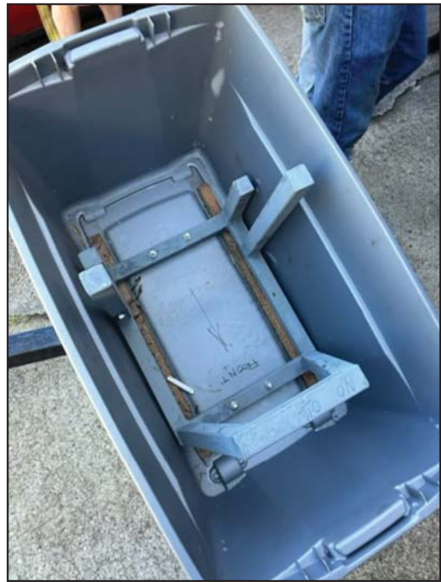
This very clever metal chassis was specifically formed to allow a ZF gearbox to be securely bolted into a shipping container. I've been waiting for years for a chance for somebody to use it!
