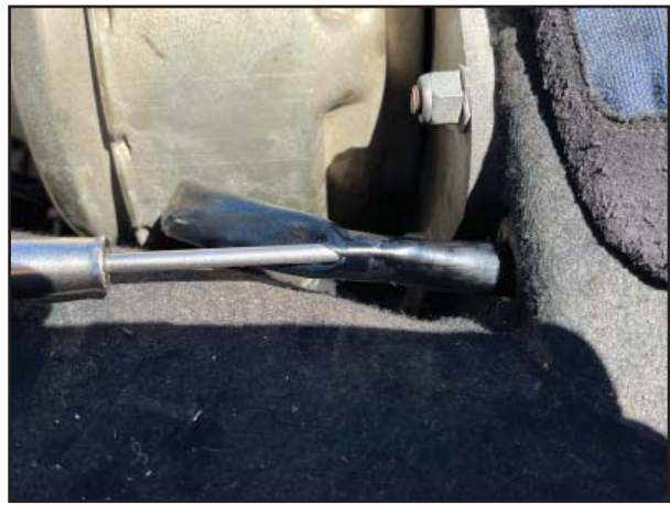
I used an awl to pierce the plastic wire bundle insulation, to give access for a WD40 spray nozzle
