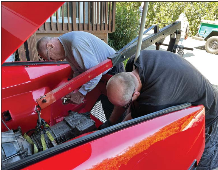
Forest and Brent set to removing the bolts holding the transaxle side mounts to the rear part of the chassis
