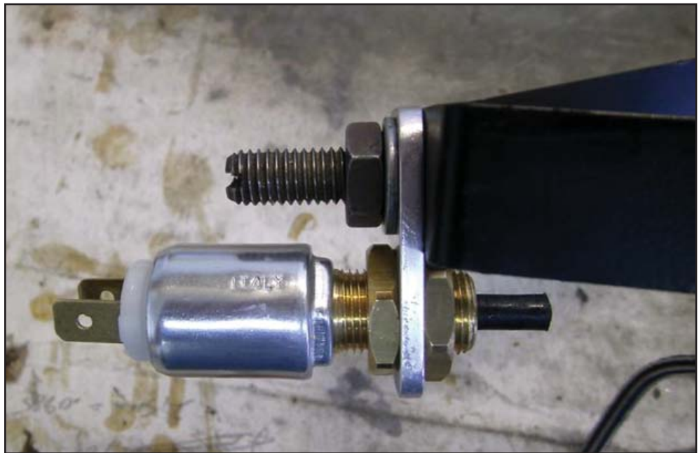
This image shows how the new switch and mounting bracket are attached to the factory brake pedal stop. The front of the car would be to the right here
