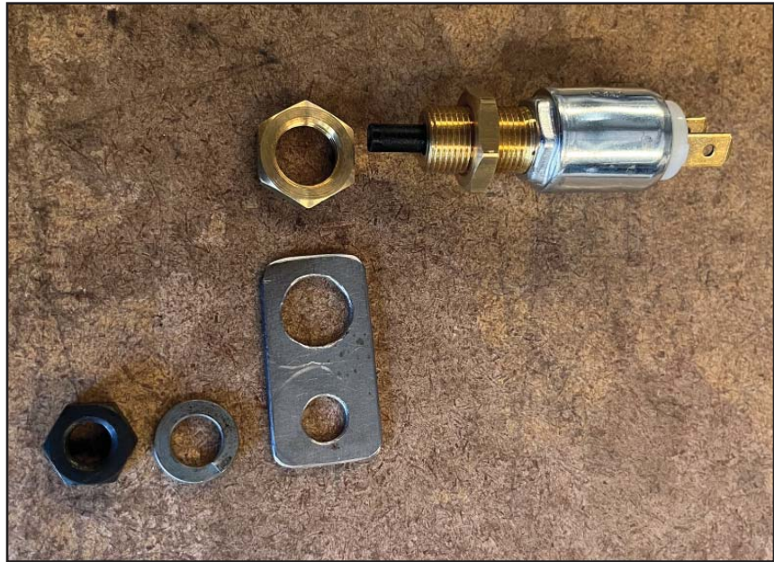
This image shows the new mechanical brake switch and the mounting bracket I formed out of aluminum
