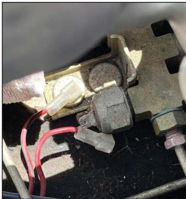
With the front of the car to the left, this shows the mechanical brake light switch, and the two small-diameter wires that need to be pulled from the front trunk to connect to the new switch under the dash
