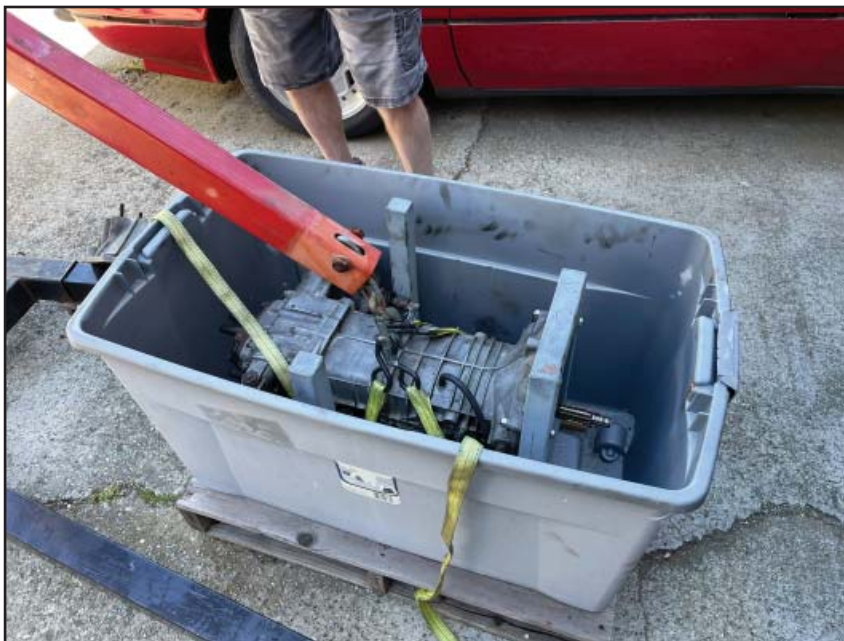
The plastic tub is watertight, but not strong. The cradle bolts through the tub onto a wooden pallet, which provides tremendous stability and security for the long drive down to Orange County
