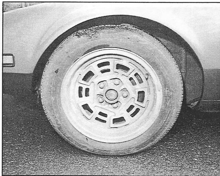
You can't run ugly, corroded wheels like this on your freshly painted Pantera! Fortunately, with some effort these wheels can be made literally better than new!
