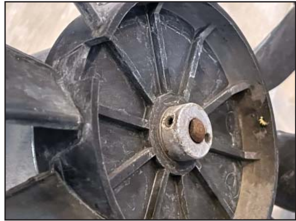
There is a notch molded into the fan blade hub that allows access to the setscrew. This notch should face the front of the radiator
