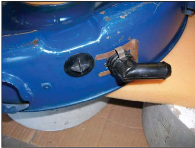
View of 71 version with plugged off "normal" position for the relocated fresh air snorkel/inlet. There is a plug in the hole for the evaporative (fumes) emission control used in CA cars. This filter may have been from a non-CA car originally. The black hose fitting and clip retains the crankcase ventilation filter (FA87), and hose from the valve cover
