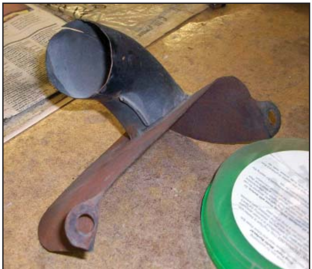
This is the special exhaust manifold heat riser for the Pantera. The Pantera MPC book incorrectly lists a standard 1971 Ford part number/piece (DIAZ-9603-A), which I have had in the past and there is no way that they are just going to bolt in place, as the part corresponding to that number was made to fit cast iron manifold. Perhaps De Tomaso cut up the original and welded it to some hand-formed sheet metal, as there are no spot welds here
