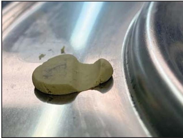
Here is result of checking the fit of WIX air filter #42113 with flat lid on one of the bases using a piece of clay. I can live with that!
