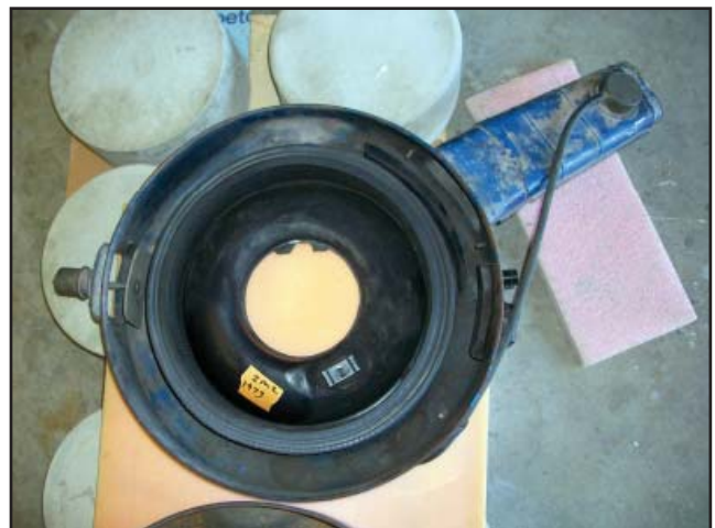
Top view of the right hand facing 1972-3 unit-auxiliary “ram air” cold air inlet with vacuum activator motor seen on left in the previous picture. All Panteras had this feature
