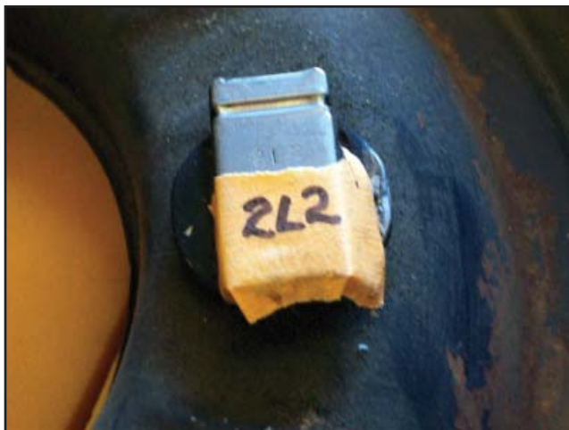
Top view picture of thermal vacuum switch to control hot/cold airflow through the snorkel during engine warm up. Sensor Assy- Carburetor Air Cleaner- Air Temp Controller: D0ZZ-9E607-B 1970+ Mustang 2L2 date code translates to 1972, 2nd of Nov produced
