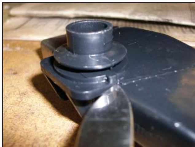
Close up picture of the tab that disappeared on some of the non-OEM "replacement" versions of the breather filter
