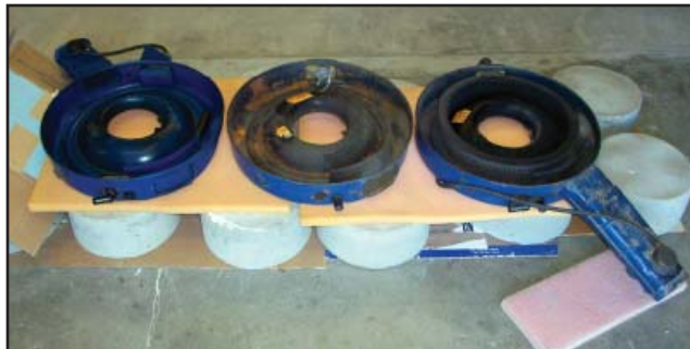
Three period Ford air filter assembly bases. The front of the vehicle would be to the right viewing these here. The one on the left is possibly a 1971 or early 1972 Pantera version. There are no dates on any pieces. The center and right hand pieces are late 1972 or early 1973 with 2L2 and 2M2 (1972 Nov and 1972 Dec) dates on the thermal vacuum switch covers. The right hand unit is from my very stock Pantera L. There are no other dates or part numbers found
