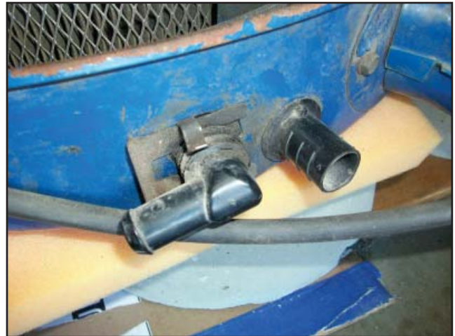
This photo shows the plastic fitting for the paper tubing that ran over to the charcoal filter affair that many have in their cars to recycle excess gas fumes from the carb.. Also black hose connection to valve cover breather filter and valve cover connection.
