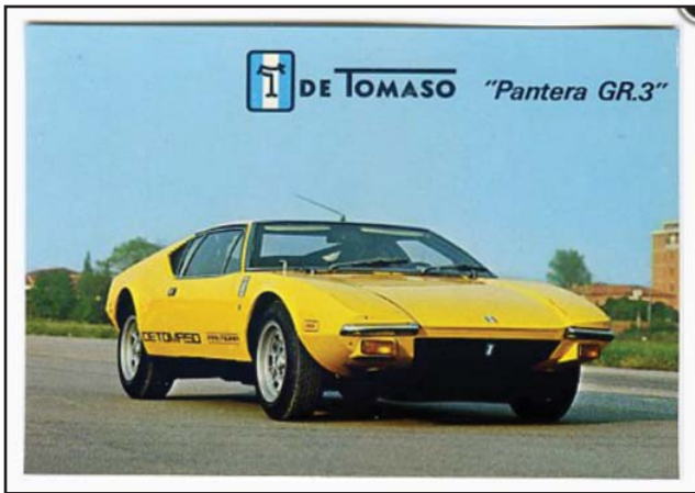
As befits its role as a race car, the factory Group 3 Pantera was built atop a standard European Pantera L rather than a higher-specification GTS. At the time, the 10-inch wheels had not yet been invented, so it wore the standard wheels and tires in compliance with the official FIA homologation paperwork. Modifications for racing include a battery cutoff switch on the top of the left front fender, unique side graphics that eliminate the "GTS" moniker, and a roll cage
