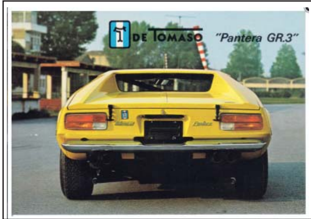
Like the Pantera L, the Group 3 race car was equipped with a one-piece chrome rear bumper. Rubber hold-downs are used to secure both the front trunk and rear decklid
