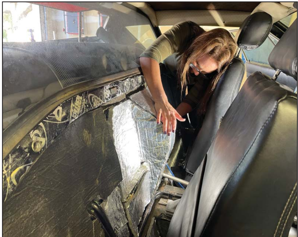
Once the easy solutions were all exhausted, we set out to check the engine timing, which necessitated the removal of the interior cover
