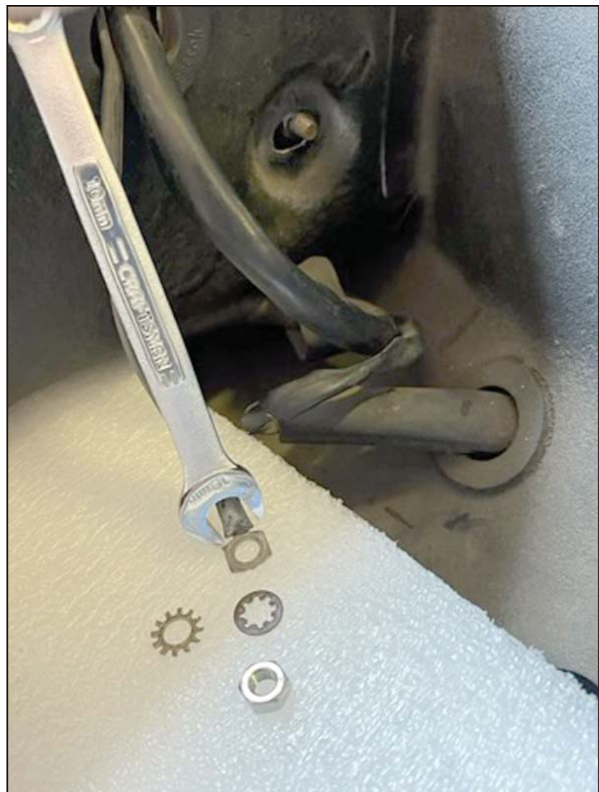
Two different styles of star washer (inside and outside teeth) are shown with the factory ground wire connector and nut. The stud in the background was clean and the paint sanded away from the body, but it was the star washers that enabled the connection to actually flow electrons
