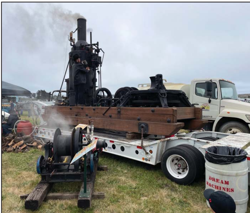
A giant steam donkey at work, with a smaller version running alongside
