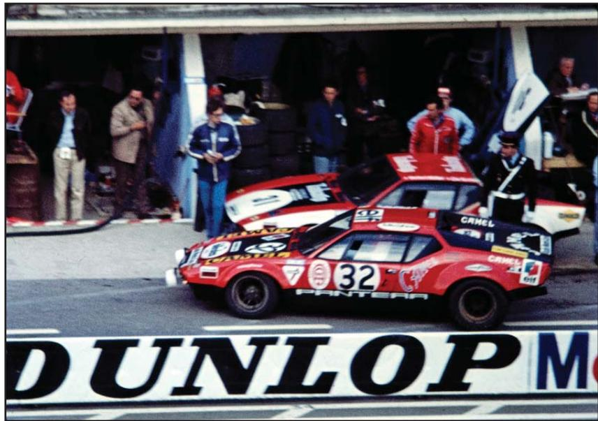
*The #32 Pantera was fitted with a very tired, bone-stock street Pantera engine just prior to the race as its race motor blew up on the dyno thanks to a balancing weight falling out of the crankshaft counterweight at high RPM, destroying the block. It was notably slower than the other Panteras, but finished the race. The mechanics of the #31 car behind are investigating the chronic overheating that was later determined to be caused by a blown head gasket*
