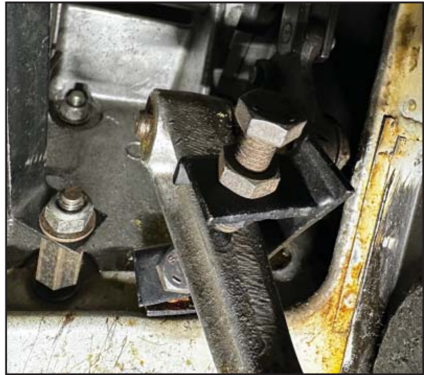
Even with the snap ring removed I couldn’t get the pedal off! It took great effort to dislodge it
