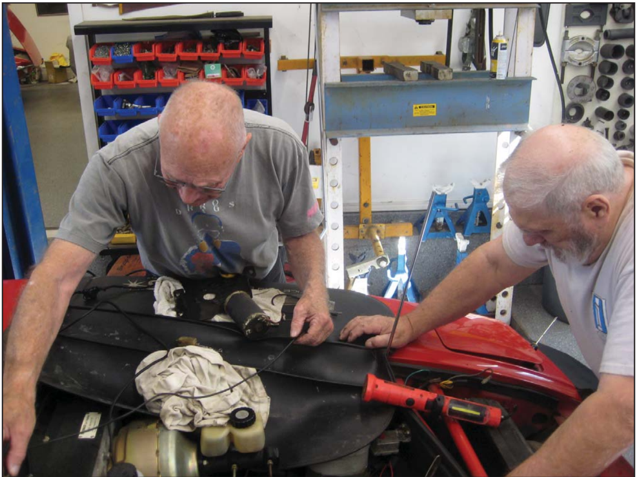
Forest Goodhart and Tom Galli worked together to find the source of the inoperative headlight raising mechanism
