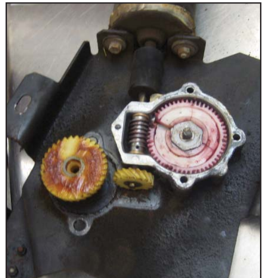
After a hard job of wrestling the window motor mechanism out of the door, Tom Leonard discovered exactly why the window wouldn't go up and down properly—a comprehensively broken plastic gear
