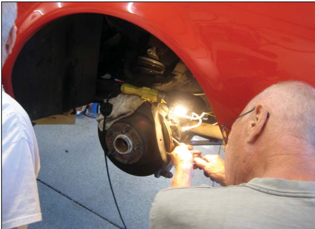
Forest later successfully diagnosed an improper brake pad as the cause of the inoperative parking brake system
