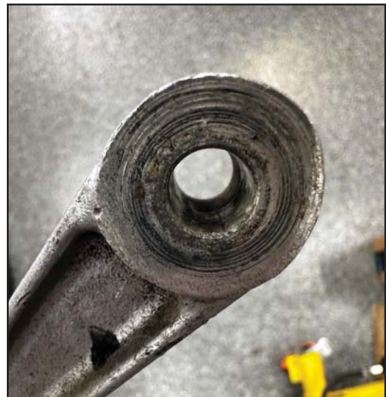
The cast aluminum pedal has a pressed-in steel insert. Post-Ford cars use a tiny roller bearing here
