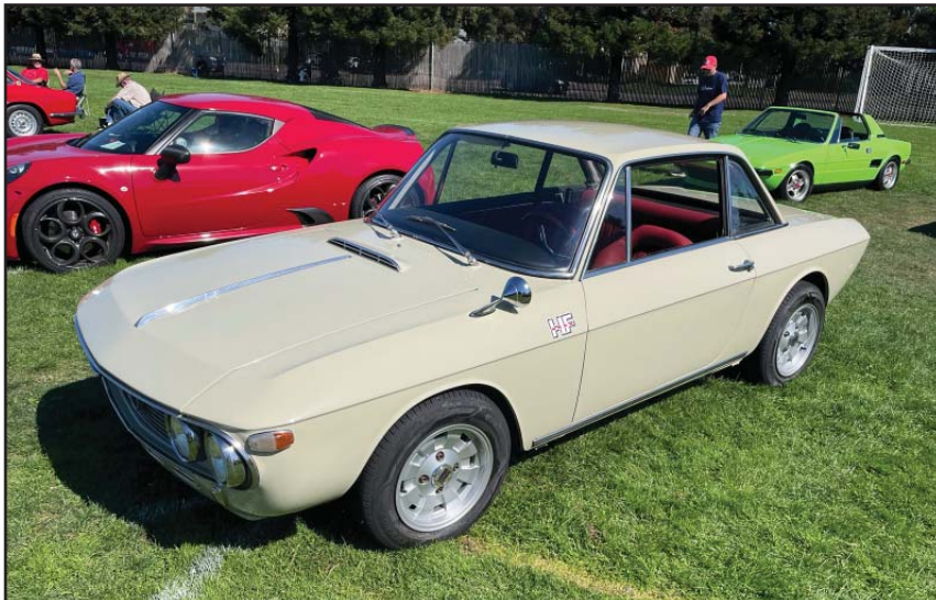
The Lancia Fulvia Coupé was an innovative front wheel drive sports coupe powered by a narrow-angle 1.3 liter V-4
