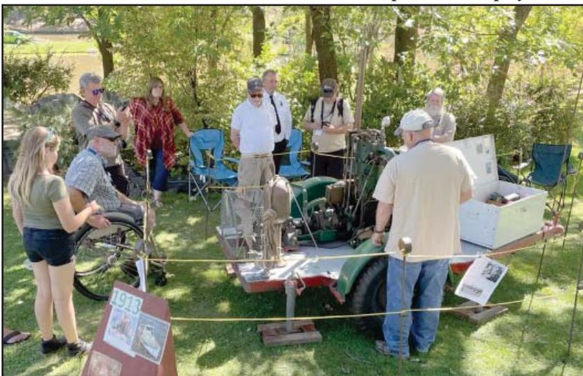
*This 1913 Hicks boat engine quietly chugged along in a corner of the show. Hicks was based in San Francisco and made thousands of robust, simple engines which powered most of the fishing boats from the turn of the century through the 1950s*
