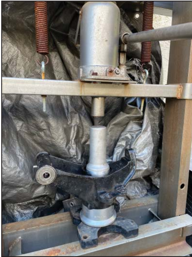
Once the axle is removed, the upright is supported on the smaller pipe and the press tool forces both bearings out
