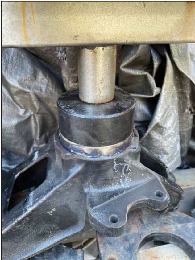
The cup-shaped tool presses the outer bearing into the upright without damaging the bearing
