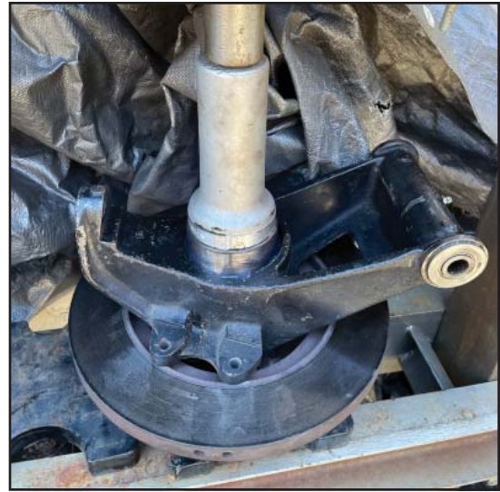
The tall press tool is hollow in the center, enabling the inner bearing to be pressed into the upright and over the axle
