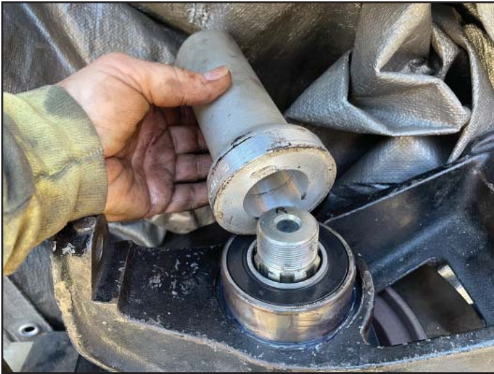
The tall press tool is hollow in the center, enabling the inner bearing to be pressed into the upright and over the axle
