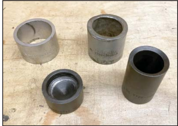
Two of these tools in the T72D-3006-A combo are used to press the ball joint out of the upper rear A-arm and the other two are used to install it
