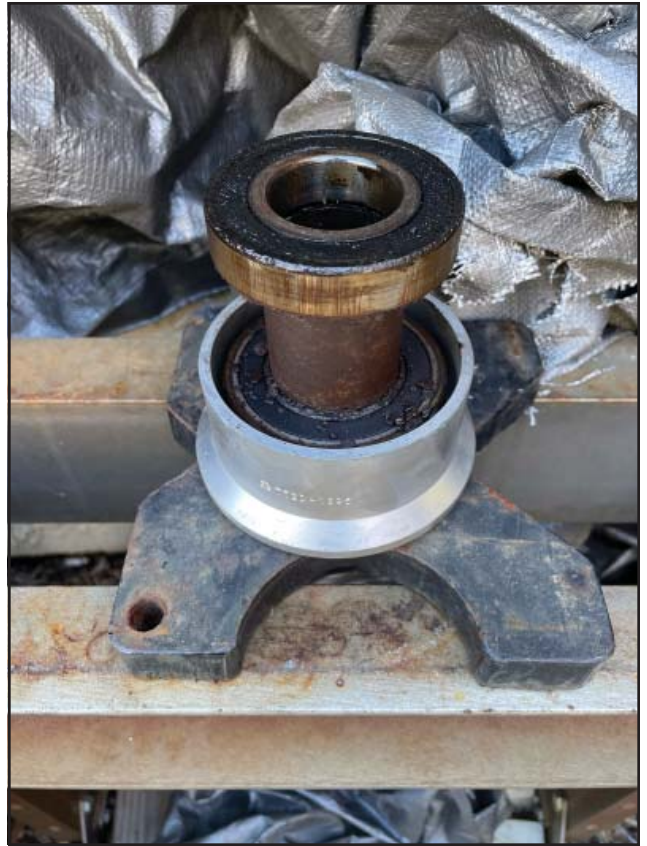
The bearing stack is left neatly standing inside the bottom tool once the upright is removed
