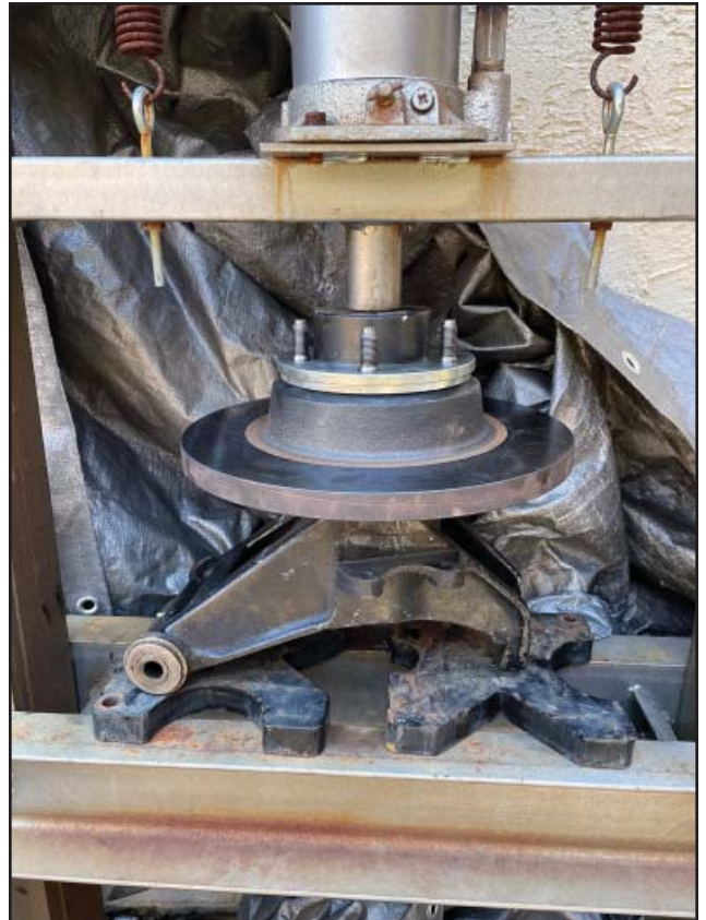
The same tool then presses the axle and rotor into the outer bearing, pressing evenly on the face of the axle
