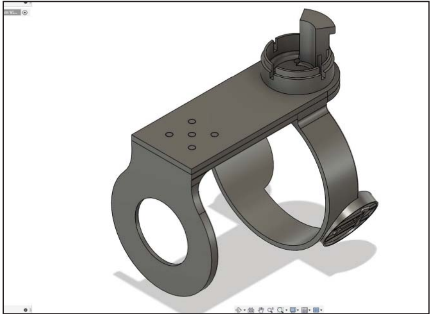
The completed 3D model of my cupholder, with the bottom to the left. The protruding hook at the top right engages with the sheetmetal skeleton in the door to hold it in place
