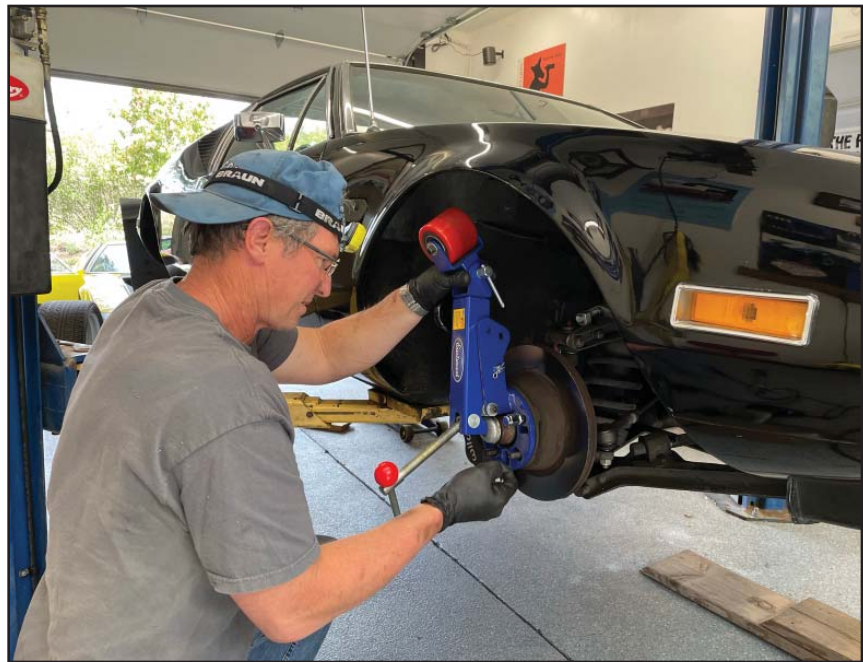
Patrick gets after his offending fenderwell lips with the help of Garth's tool
