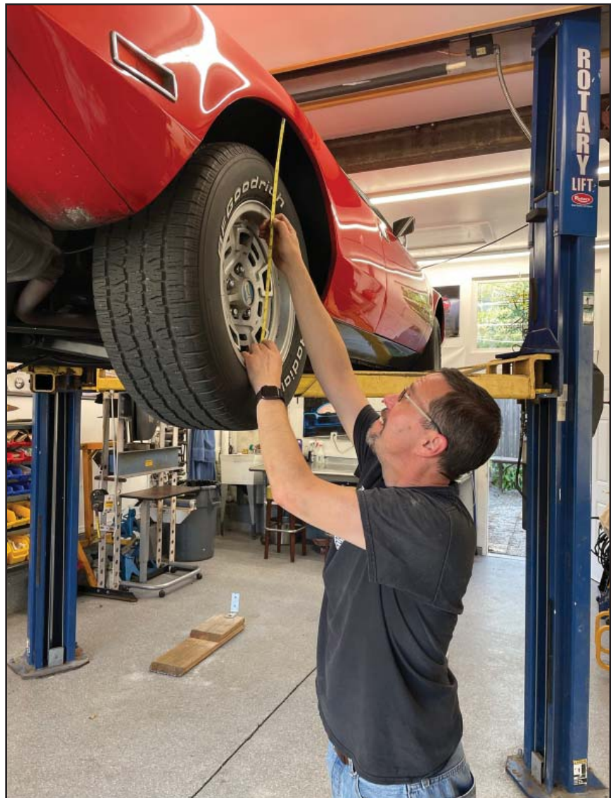
John Mardesich attempted to establish a baseline on Paul Fahndrick's suspension by measuring from the top of the fenderwell to the bottom of the wheel on each side of his Pantera. Not surprisingly, all four corners were different from one another. In the end, the decision was made to simply raise both sides an equal amount on the rear, which resulted in a notable handling improvement
