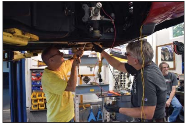
It was a team effort as Mike, Forest and Paul worked together to reinstall the rack in Paul's Pantera. Once that was done, it was time to turn to plumbing the new brakes
