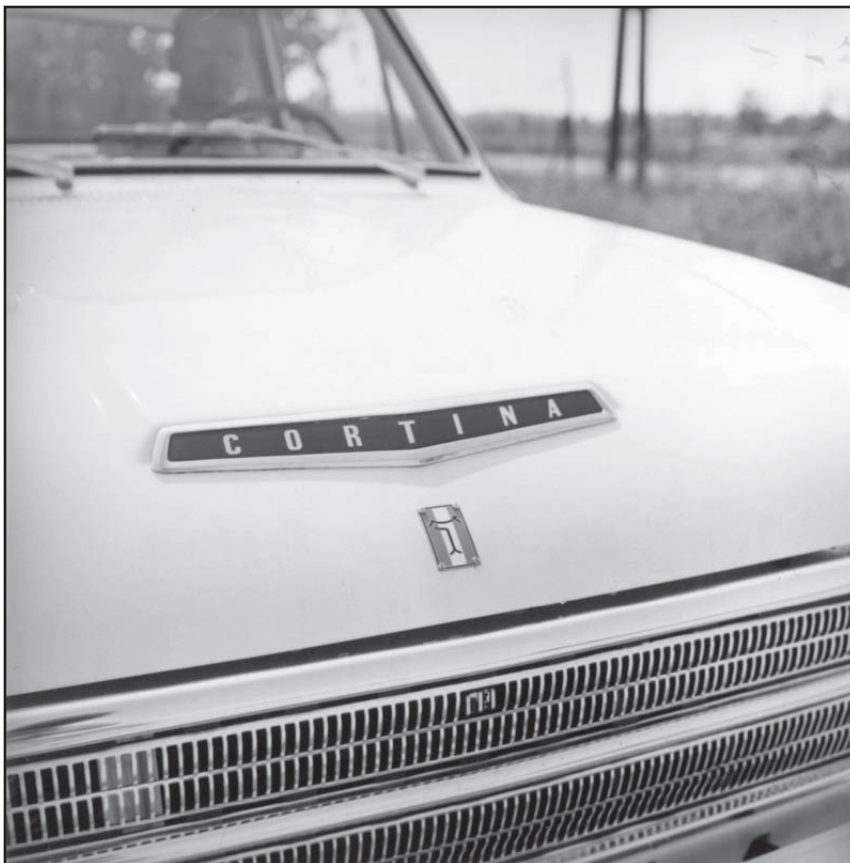
Note the De Tomaso cloisonné logo, which was bent to match the contour of the hood and then crudely secured with four screws
