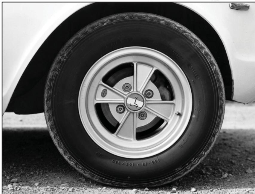
The De Tomaso Cortina GT used these unique Campagnolo wheels. Note the use of the early De Tomaso wheel center emblem, which had the Argentinean flag laid out horizontally instead of vertically behind the De Tomaso crest
