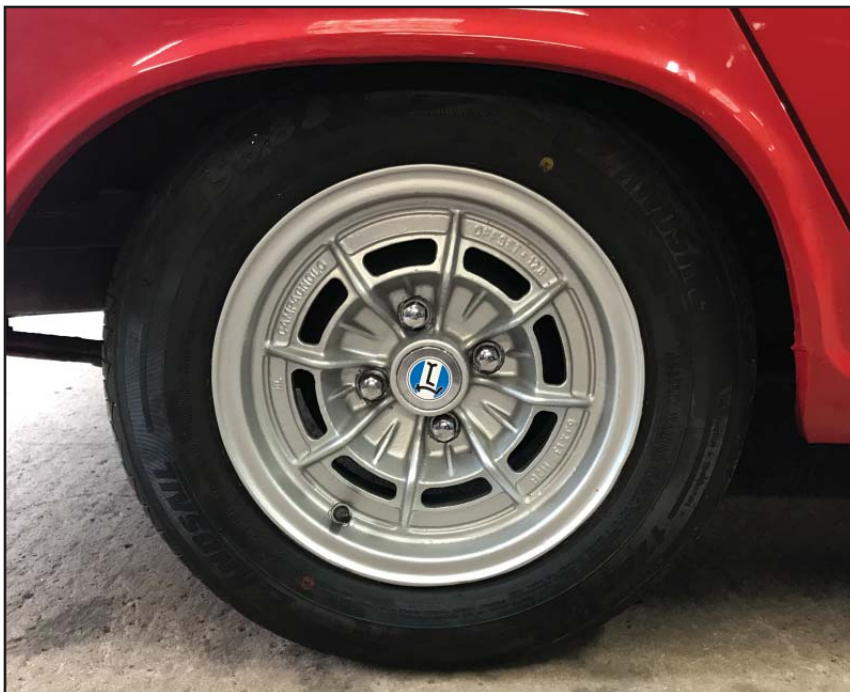
The wheels were intriguing. Although not the same as those on the known De Tomaso Cortinas, they were a rare Campagnolo Elektron (magnesium) design that De Tomaso had used on other cars. However, these wheels were date-stamped as having been manufactured in 1973....
