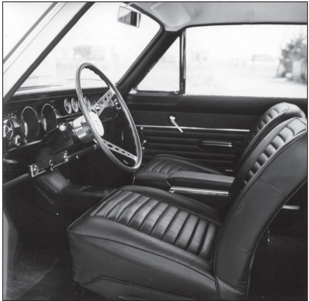
Among the interior features unique to the De Tomaso models were the British Les Leston steering wheel, and the Italian Brev Lanz seats
