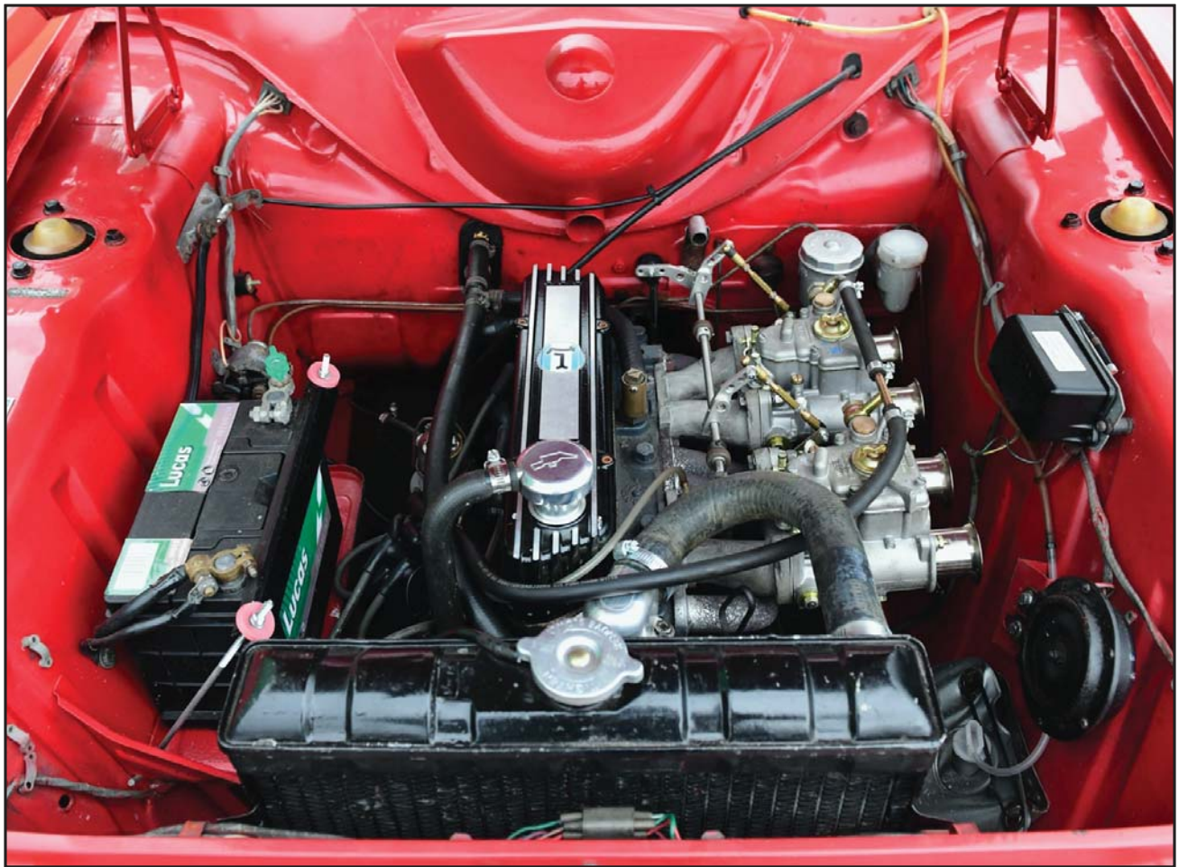
The engine bay is nicely detailed, but the valve cover is incorrect. Instead of the beautiful cast De Tomaso cover as used on the Vallengunga, this is a generic aftermarket cast cover with an ordinary De Tomaso sticker glued to it!
