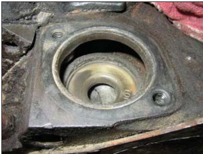
This radiused brass disc pressed into the top of the block is a critical component of the 351C cooling system. Eliminating it or using the wrong thermostat leads to chronic overheating, and blocking it is harmful too
