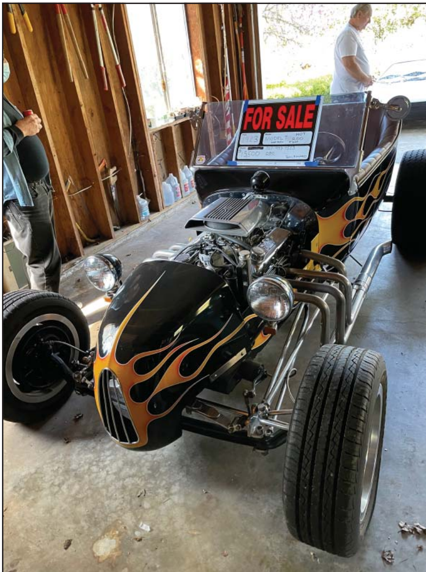
Tom's 1923 T-bucket generated a lot of interest, as it is a car completely outside the experience of most of us. It's an all-steel, original 1923 Model T with a custom nose, powered by a pumped-up Ford 302. It has proven sufficiently powerful to rip the rear suspension right out from under itself!
