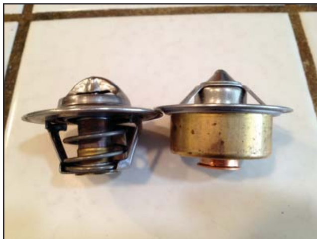
Both of these thermostats are intended for the 351C. The one on the left is a standard unit, costing less than $10, while the one on the right is the FlowKooler Robershaw High Flow unit, which is more like $45
