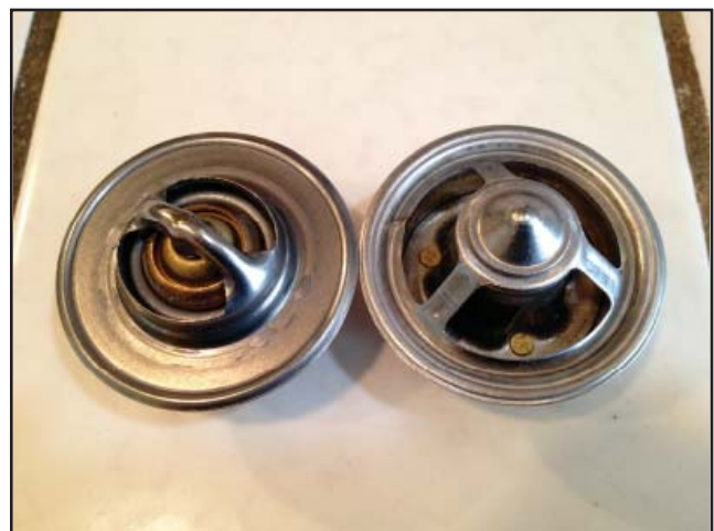
Both of these thermostats are intended for the 351C. The one on the left is a standard unit, costing less than $10, while the one on the right is the FlowKooler Robershaw High Flow unit, which is more like $45
