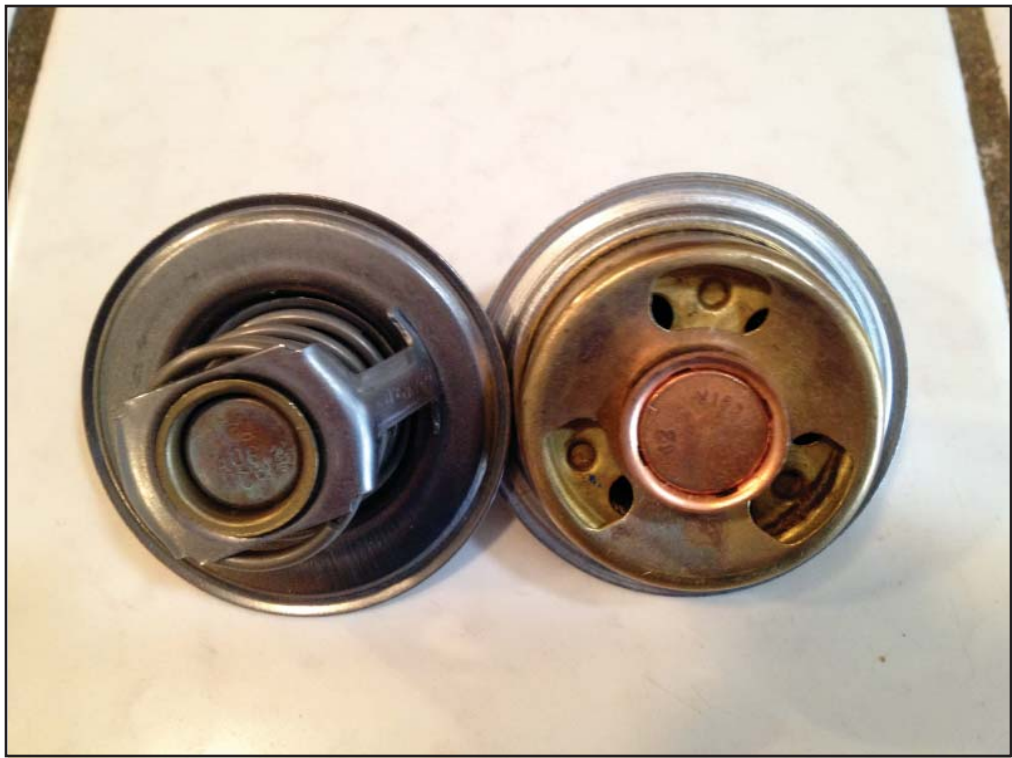
The business end of both thermostats, showing that the pressed-on 'hats' are identical in diameter
