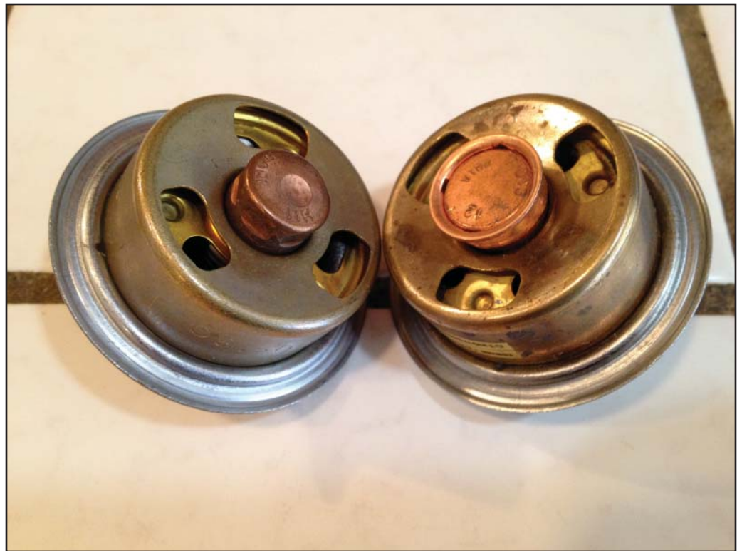
A high-flow thermostat for a regular Ford engine appears on the left, and a specialized 351C thermostat on the right. The only difference between them is the brass 'hat' pressed onto the end of the thermostat, which serves to more completely block the orifice in the disc pictured earlier
