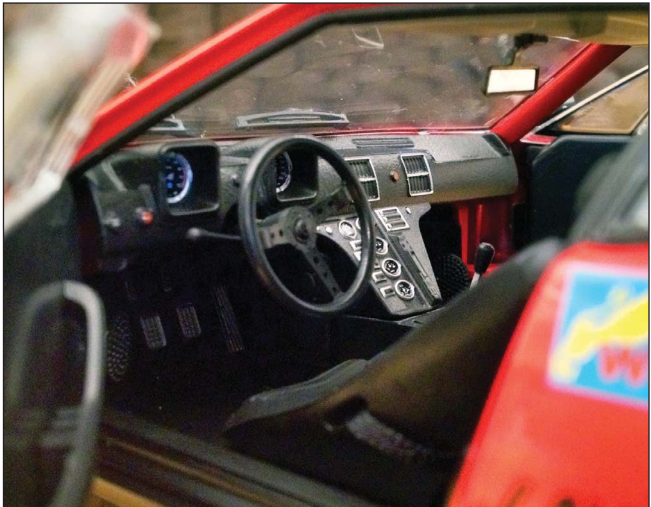
The level of interior detailing is almost absurd! Notice the numbers on the speedo and tach, as well as the De Tomaso logos on the main instrument faces. The minor gauges, switches and heater controls are all replicated accurately, as are the pedals. The steering wheel accurately copies the three-spoke Momo Prototipo used on the original car as well
