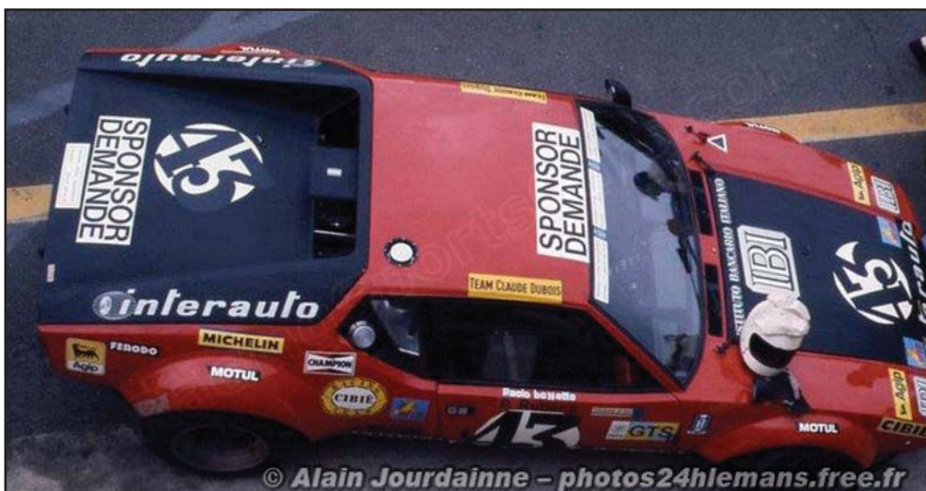
This unusual overhead view shows some of the unique details of the factory Gr4 cars as they evolved over the years. The fuel tank (which was on the right side) originally used a Cobra-style flip-cap in the side gill, but by 1975 changes in the regulations meant it was converted to a dry-break filler in the roof with a side vent. Also note the air scoop/rain shield over the Webers
