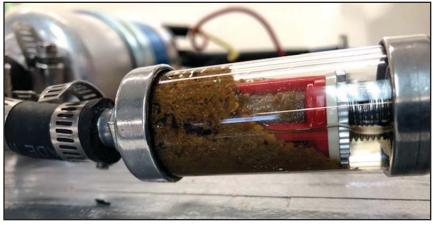
The fuel filter was completedly clogged after only three minutes! It required multiple iterations of sweeping and filter cleaning before he was done
