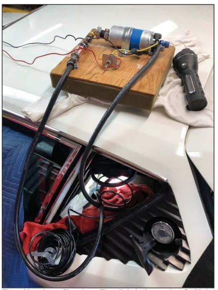
The tool in action on Shawn's car. The coiled wire is a very long flexible borescope camera
