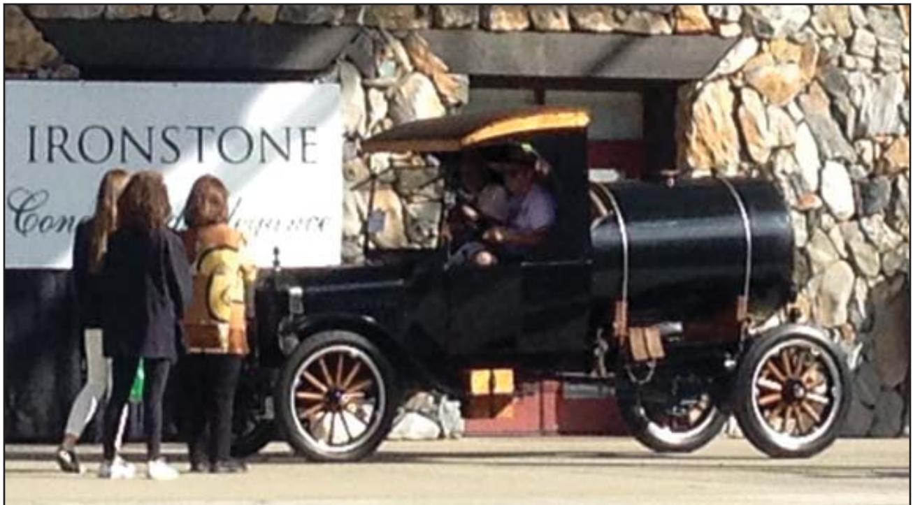
Best of Show went to this 1923 Ford Model TT 1-ton tanker truck. With standard gearing a TT could only achieve 15 mph, and with the optional high-speed gears, it could hit a whopping 22 mph!
