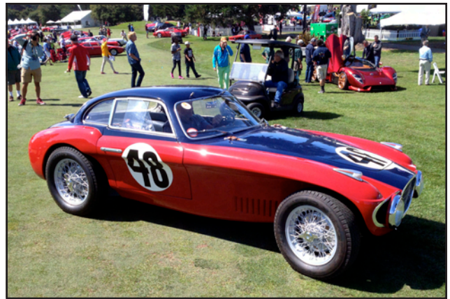
This remarkable 1952 OSCA MT4LM features a body designed by Giovanni Michelotti, and built by Vignale. It used an aluminum 1.3L DOHC four, producing 96 hp
