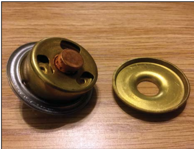
The new Robertshaw 333-180 thermostat is actually a Windsor 330-180, with a new disc included in the box
