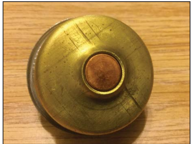
The hole in the disc is much smaller than stock and is completely blocked, which means that if the thermostat isn't perfectly centered it won't work
