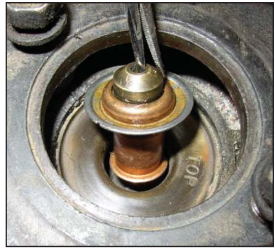
This partially dismantled 351C thermostat clearly shows the relationship between the outside of the hat, and the hole in the center of the disc
