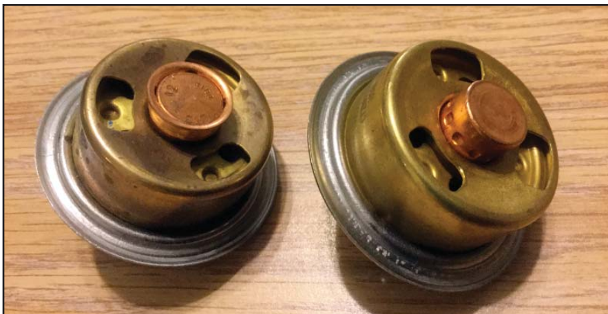
The original (and proper) 351C Robertshaw thermostat on the left, and the 351W unit sold as part of the new 351C 'kit' on the right
