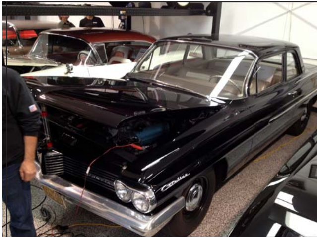
Super Stock drag racing was a big thing in the early 1960s, with all the manufacturers building special lightweight versions of their production sedans, equipped with ever-more-powerful big-block engines, aluminum bodywork and bumpers, thinner glass, and with fripperies such as heaters, insulation, carpeting and so forth deleted. On the left is a 1962 Pontiac 421 Super Duty, and on the right the competing 1962 Cheverolet 409
