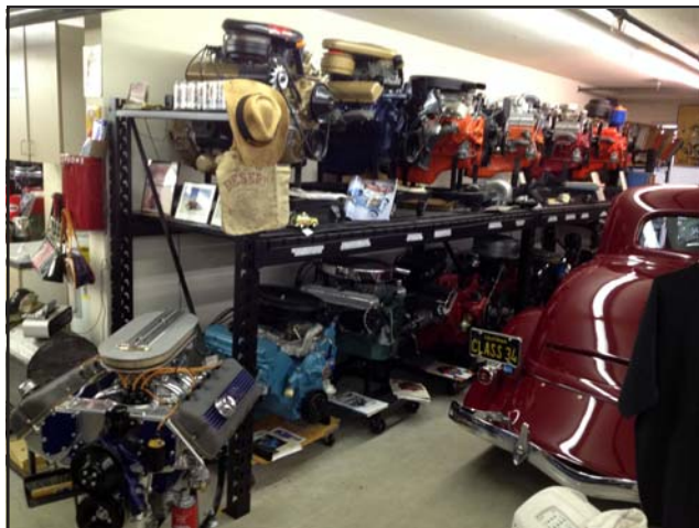
A corner of the Ford building was dedicated to a collection of ultra-high-performance Ford engines, with the most significant being the 427 Single Overhead Cam (SOHC). Designed to compete in NASCAR, and immediately banned, it features iron heads with mirror-image overhead camshafts, driven by a timing chain that is nearly seven feet long! It saw great success in NHRA drag racing
