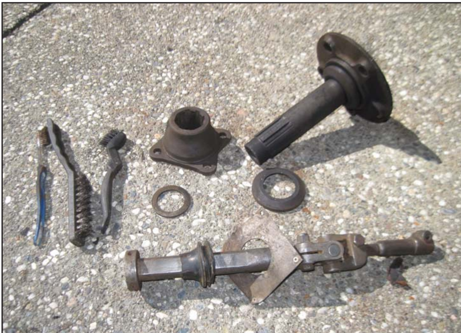
Just a few minutes work with a hose, followed by metal brushes and a toothbrush, resulted in parts that looked as good as new. Those that were originally coated in black oxide (which itself is a form of rust) were left very black, while parts that were originally just bare steel had a lighter coating of black
