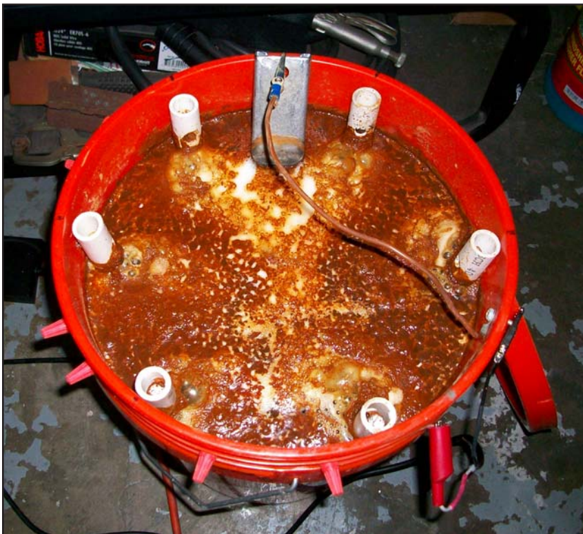
The system in action! A nasty slurry of rust and hydrogen bubbles to the top, and with time, eventually the rust particles settle to the bottom. The seat track has already been treated on the visible end, then flipped over so the remaining portion can be treated
