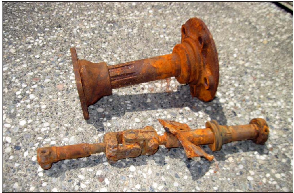
A plastic bin full of Pantera parts was left outdoors and developed a leak, which allowed it to fill with rainwater, causing the rust seen here. This would be a great test for the effectiveness of this system
