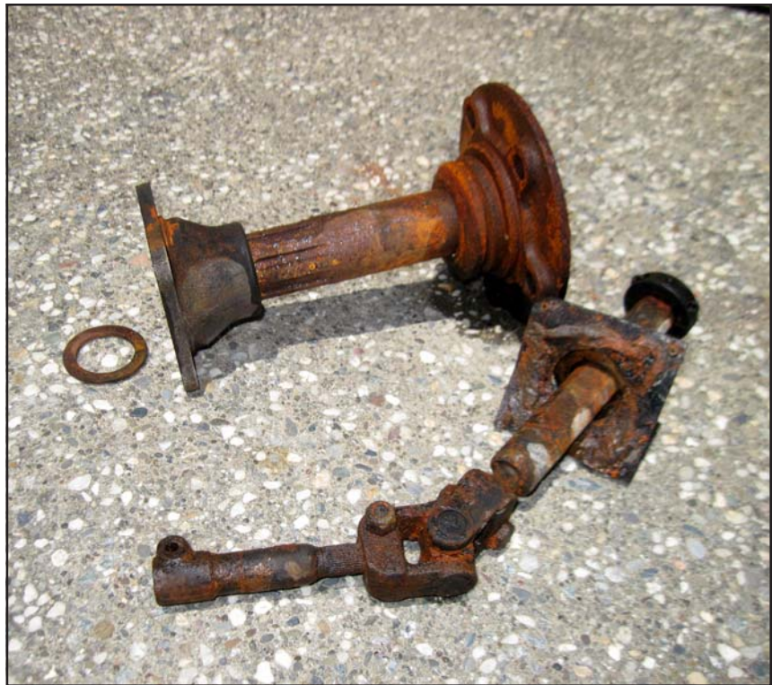
After several hours in the bath, the parts emerged looking like this. At first glance this is not encouraging, but the rust isn't actually adhering to the parts any longer; it's just sitting there, resting on the surface
