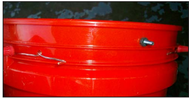
The outside of the bucket, showing the protruding end of the ground wire bolt on the right, and the first of the rebar wires for 12V on the left
