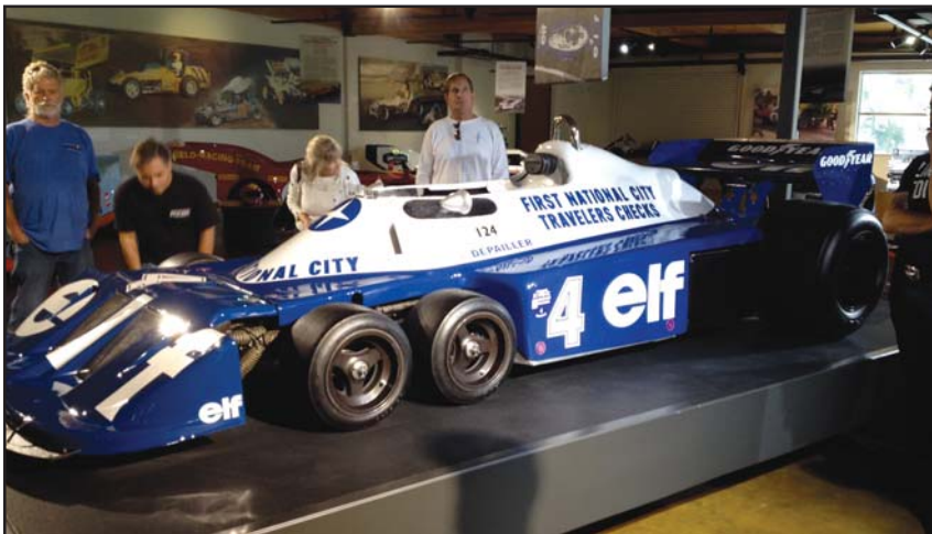
The legendary 1976-77 Tyrrell P34 six-wheeler Formula 1 car was an innovative design, using four smaller front wheels to lower overall drag and improve speed on straights, and clean up the aerodynamics so the rear wing would receive cleaner airflow. It always struggled to be competitive, and ultimately it proved to be an engineering cul-de-sac and the idea was abandoned
