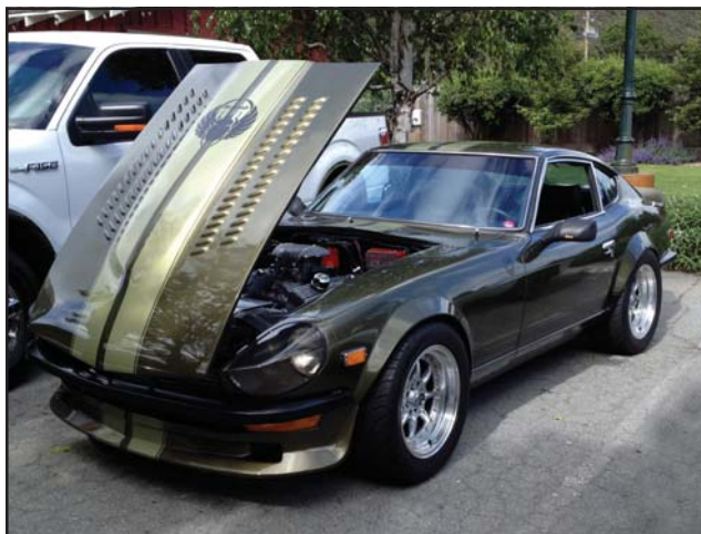
Few people have ever seen a genuine Scarab, but there was one at Baja Cantina! A few hundred were built in the 1970s by stuffing a Corvette V-8 into a heavily beefed-up Datsun 240Z. The resultant car would easily eat a Pantera's lunch!
