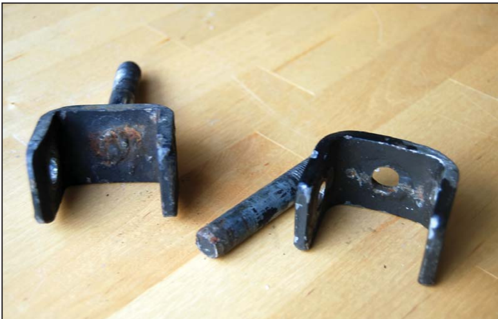
The broken (rearmost) yoke on the right, with the not-yet-broken one alongside. Note that there is rust evident in the weld between the shaft and the stamping, which might have contributed to the failure of the other one
