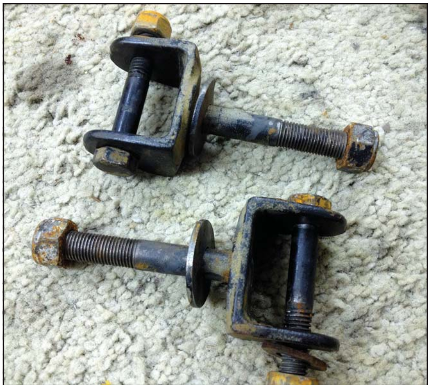
The yokes taken from a 1973 Pantera appear to be substantially stronger than the earlier style
