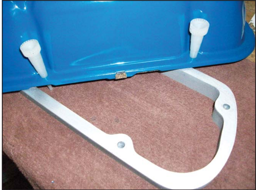
The valve cover rests atop the spacers simply to show how the ends of the caps protrude through to act as centering devices for the gasket beneath
