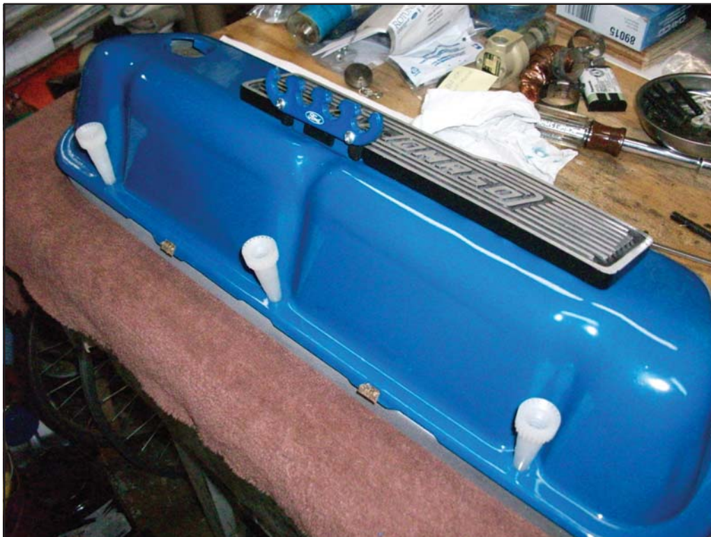
The valve cover placed atop the spacer, which provides even pressure all the way around the valve cover. Since few people have spacers lying around, one could easily use an old cylinder head, or even the heads that are on the engine
