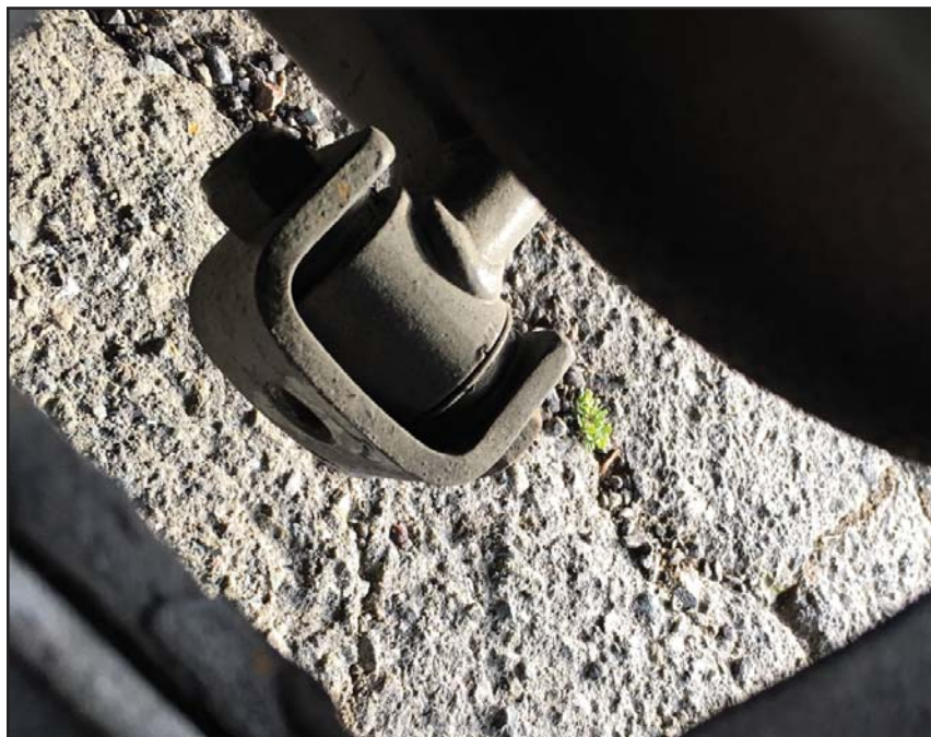
Looking down through the chassis, the A-arm and broken mounting yoke can be seen resting on the ground
