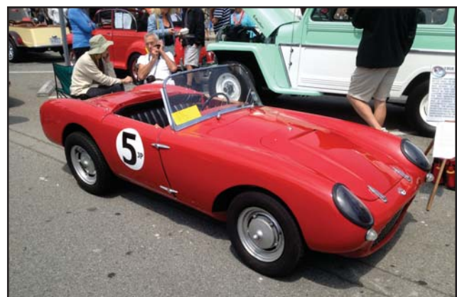
The 1958 Berkeley SE328 has a 328cc two-stroke engine powering the front wheels; this one has SCCA race history
