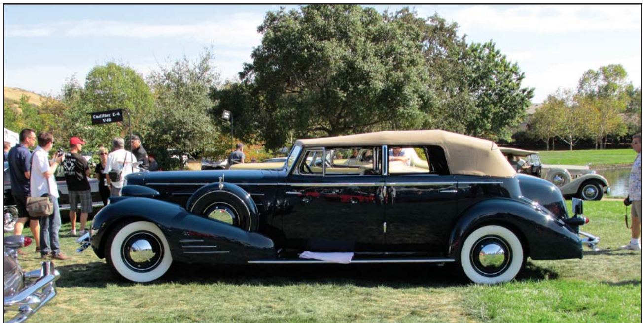
In the 1930s, big cars were BIG, like this Cadillac Series 452D four-door convertible. It is propelled by a 452-cubic-inch V-16. It only had 5.3:1 compression so it only made 165 hp, but it had tons of torque and incredible smoothness
