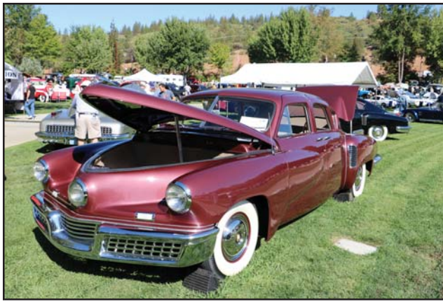
The Tucker 48 was a cutting-edge design, easily ten or twenty years ahead of its time. Sadly the company was underfunded (and some say the victim of a conspiracy by the Big Three domestic automakers) and only 51 were built. The flat six engine was a modified Franklin air-cooled helicopter engine, converted to water cooling
