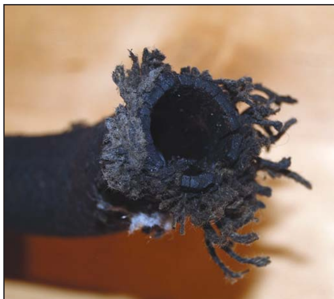
While the clearly visible portions of Lori's vacuum hose looked okay, lurking out of view was evidence of dramatic failure. Don't let this be you!
