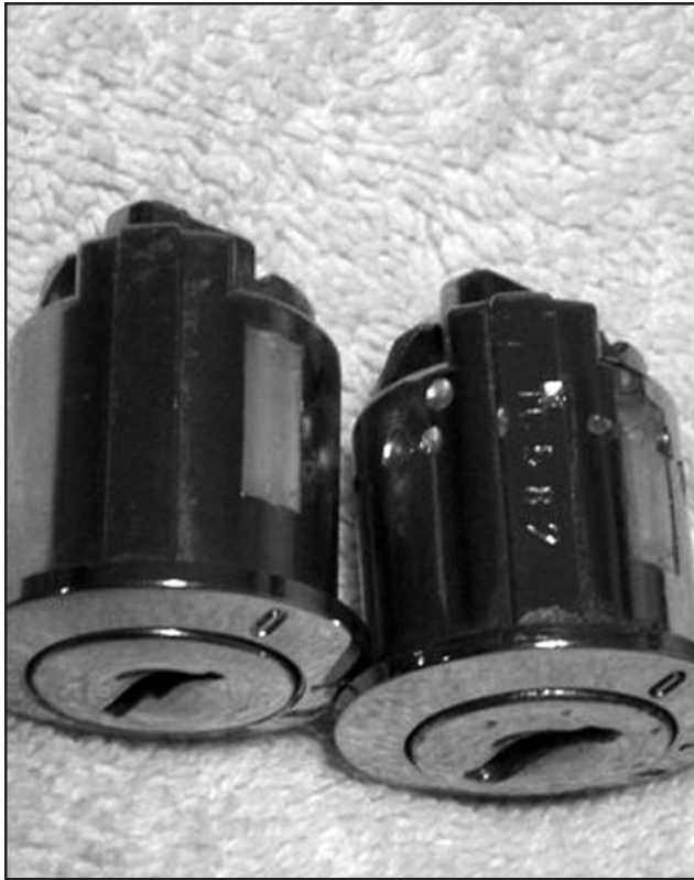
Here are two tumbler assemblies. Note that the one on the left has no number stamped on it.
