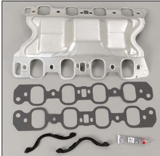
The stock-style valley pan gasket has an unfair reputation for leaking, but if installed correctly, it's a superior solution
