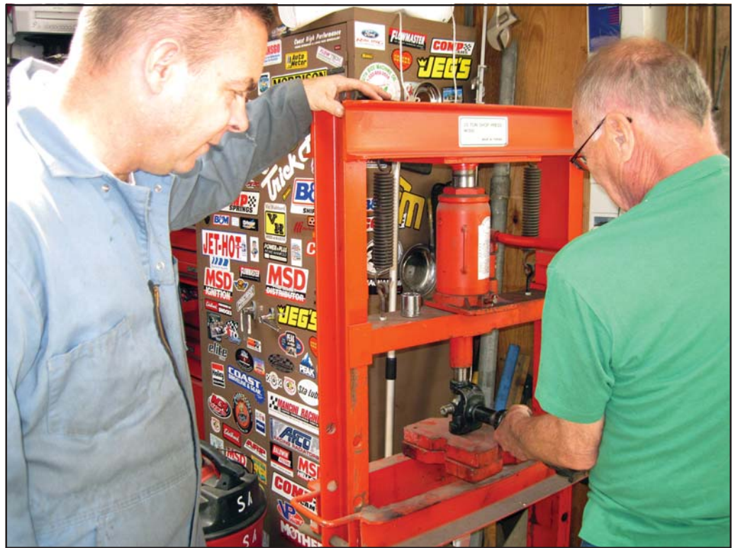
It was a valiant effort, but ultimately the attempt to rebuild Mike's driveshafts proved fruitless, as U-joint caps broke left and right!
