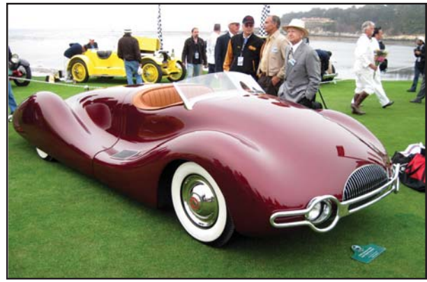
The 1948 Norman Timbs Emil Diedt Roadster was a one-off mid-engined car powered by a Buick straight-8. Designed and built by a mechanical engineer right after WWII, it featured a one-piece hinged rear body which raises to expose the engine. The body was fabricated in aluminum entirely by hand; the car took two years to build and was featured on the cover of Motor Trend
