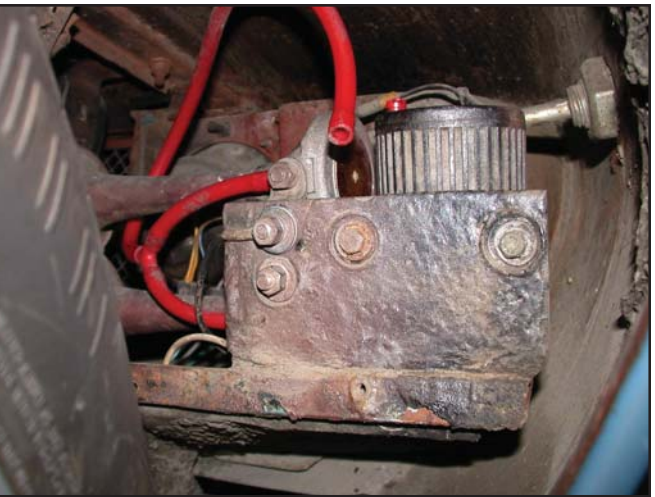
Installed ahead of the right front wheel, the air horn system is completely hidden behind a splash shield
