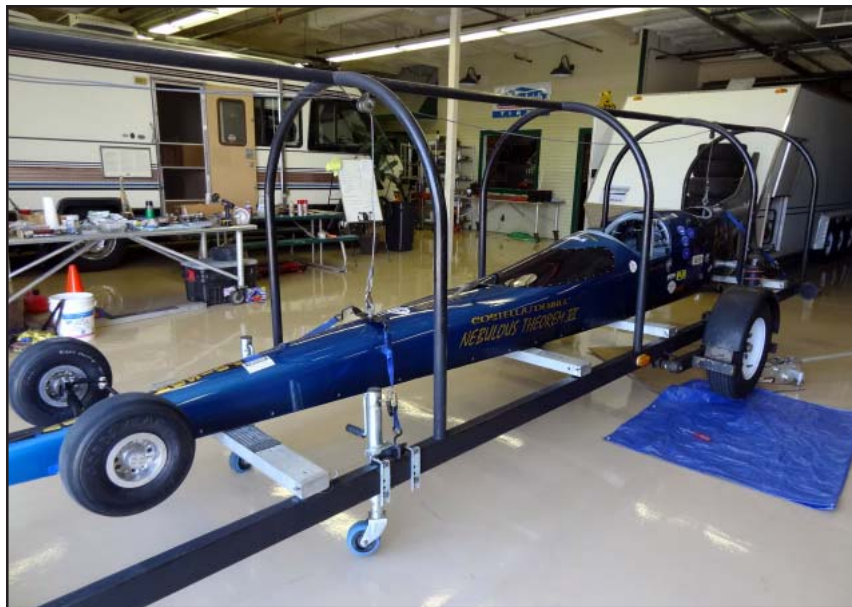
Nebulous Theorem VI is technically a lakester, not a streamliner, due to its exposed wheels. It also holds several land speed records
