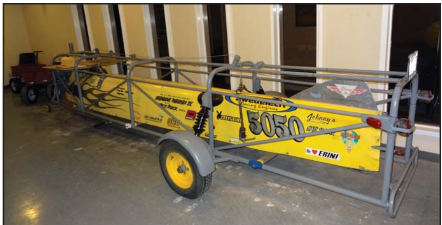
Glen's true passion was for streamlined land speed racers. He built exoskeleton trailers to haul them to Bonneville and El Mirage. Nebulous Theorem IV addressed the issue of reducing frontal area by positioning the driver on his stomach, facing forward, Superman-style
