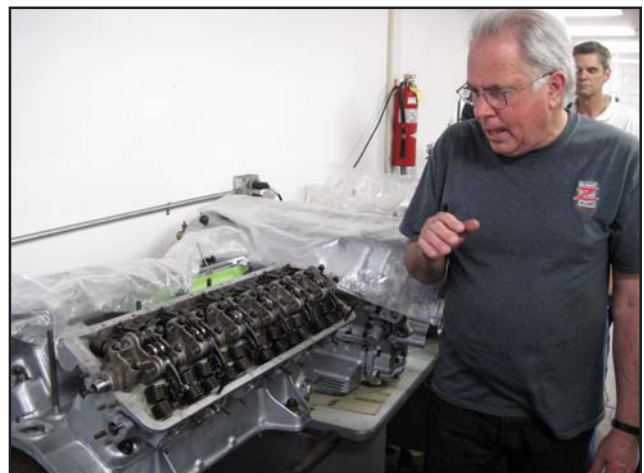
Patrick went into great depth, explaining the inner workings of a 60-year-old Ferrari V-12. Of particular note were the multiple hairpin valvesprings for each rocker arm
