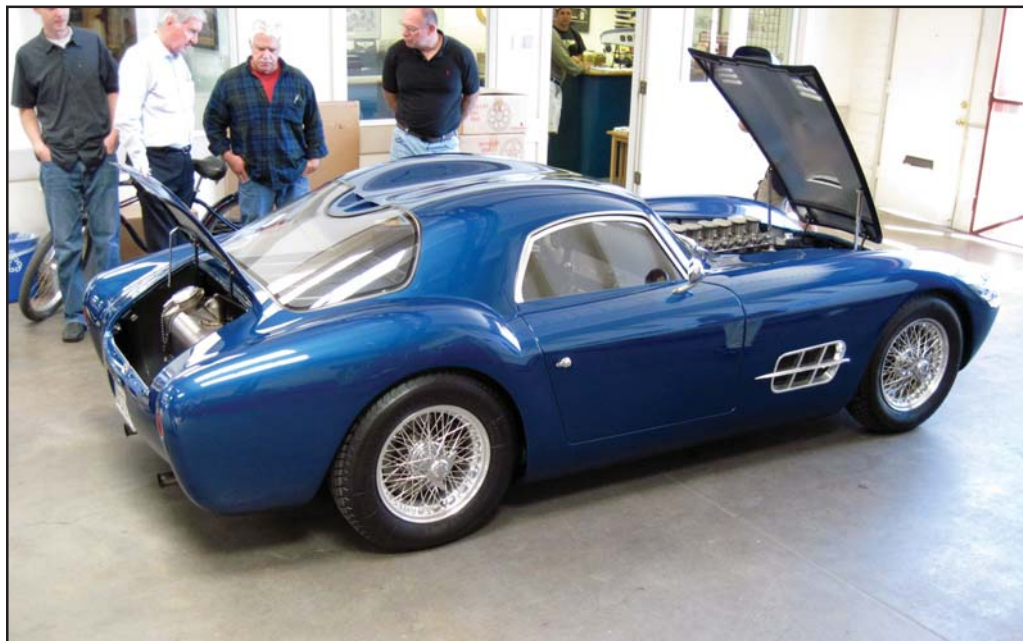
The Gatto is a Moal creation which pays homage to the great Zagato designs of the past. With shades of Maserati A6GCS/54, it features a Ferrari 330 V-12 engine and running gear, but the chassis, body, glass, fixtures, interior etc. are all hand-made one-offs
