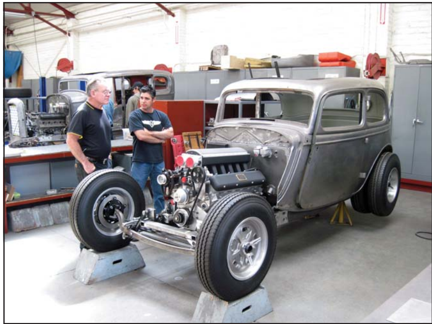
Moal's latest creation is a super-street-rod, powered by a $75,000 Falconer V-12, and using a dually rear axle with Halibrand knock-off wheels
