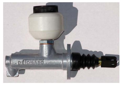
they didn't run DOT 4 fluid; that is patently untrue, because DOT 3 and DOT 4 are interchangeable and are the same except that DOT 4 has a higher boiling point. Since there is no heat associated with clutch operation, either fluid should work well.
