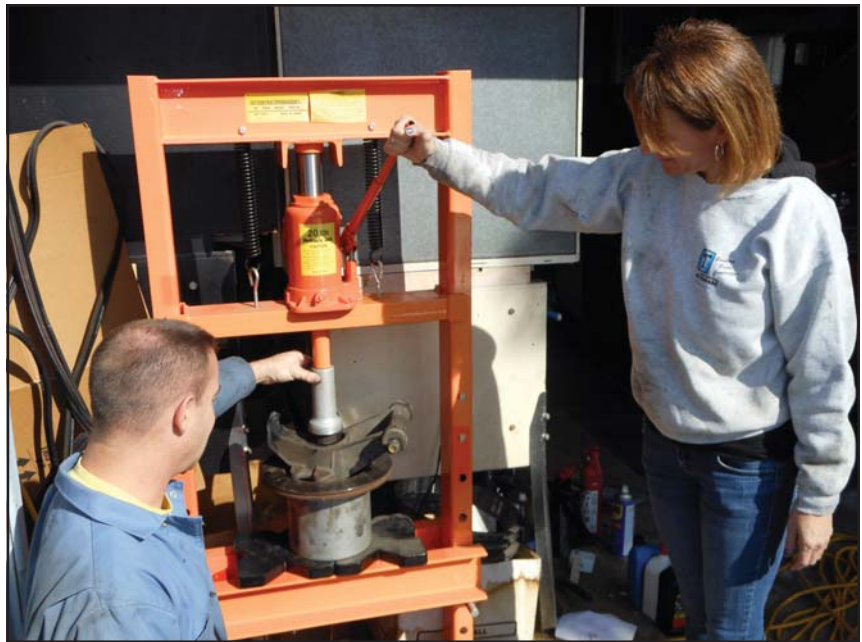
The day got off to a good start, as Ron Southern's axle proved unusually cooperative. Here Lori Albino presses the assembly apart with Mike Drew's help
