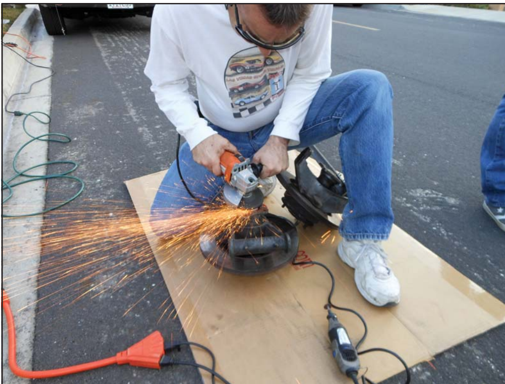
Mike got down to business with an angle grinder, and later a Dremel tool with a cutoff wheel, to carefully cut away the weld and allow the nut to be removed—or so you would expect...
