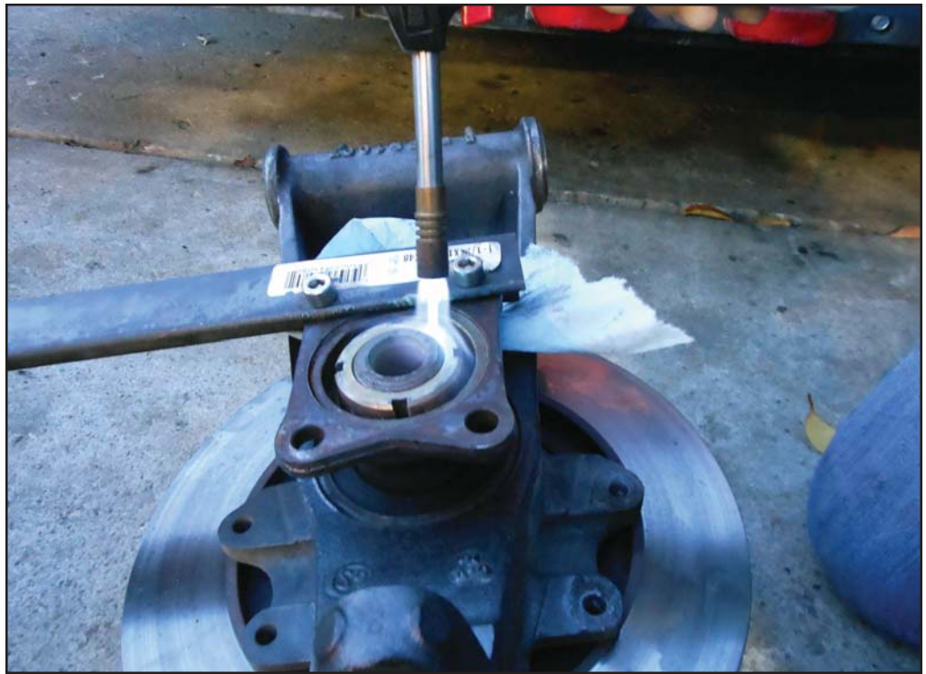
We finally had to resort to the blue-tipped wrench to melt the Lok-Tite; the 500-ft/lb impact gun then showed this nut who's boss!
