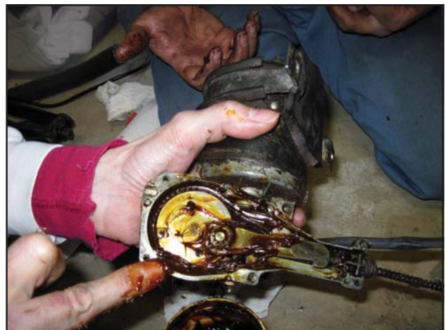
The problem was caused by corrosion inside the case, and hardened, dried-out grease. Here it gets fresh lubricant
