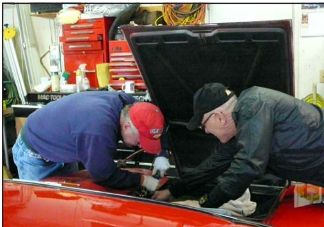
Garry Choate and Ron DeMaderios wrestled with the new master cylinder; the booster pushrod needed to be shortened
