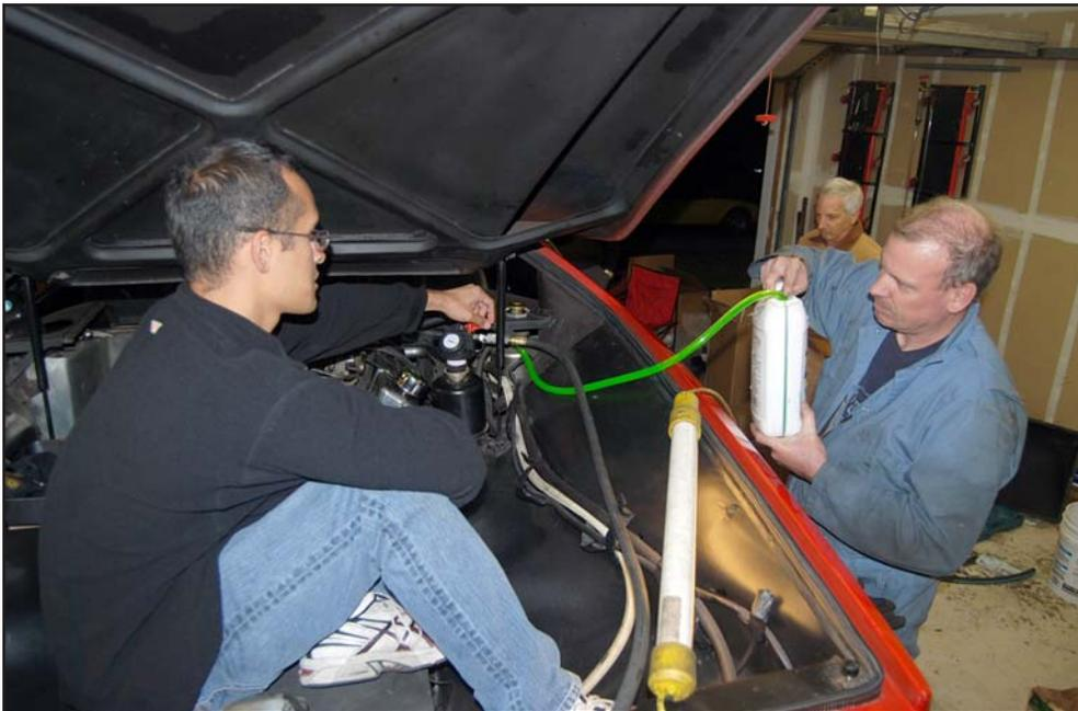
*Kaizer and Julian worked together to effortlessly fill the cooling system using an incredible device that relies on vacuum generated by a standard air compressor; it eliminates all air in the system, and hence all need for bleeding!*
