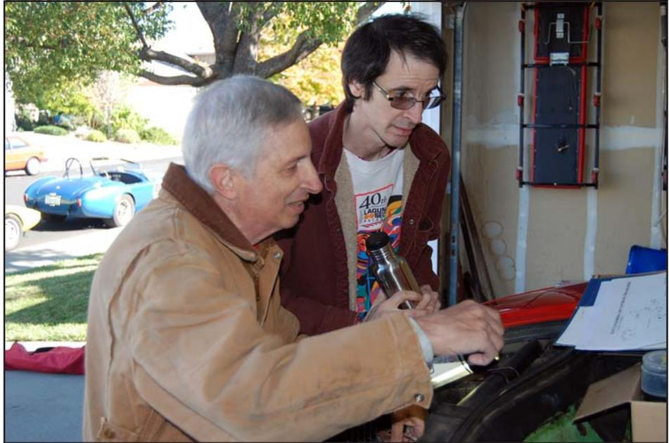
*With the radiator removed, Jim Seiferling and Mike Haney worked on straightening out the wiring and fixing the radiator fan and headlight circuits*
