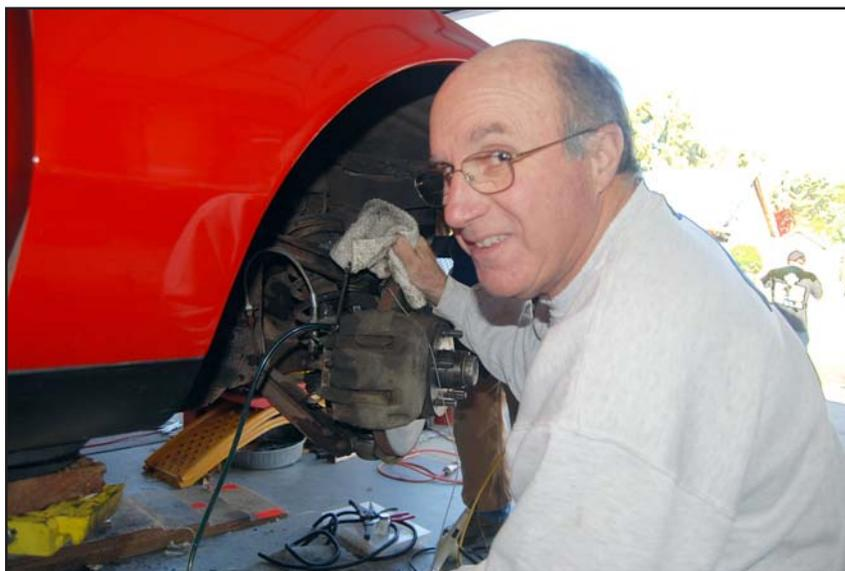
*Steve Dalcino installed new braided steel brake lines, then bled the brakes with Mike's pressure bleeding system*
