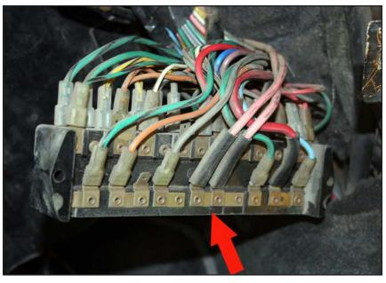
The arrow points to a tiny burn mark on the plastic body of the fusebox, caused by the fusebox cover bolt touching the unfused power strip
