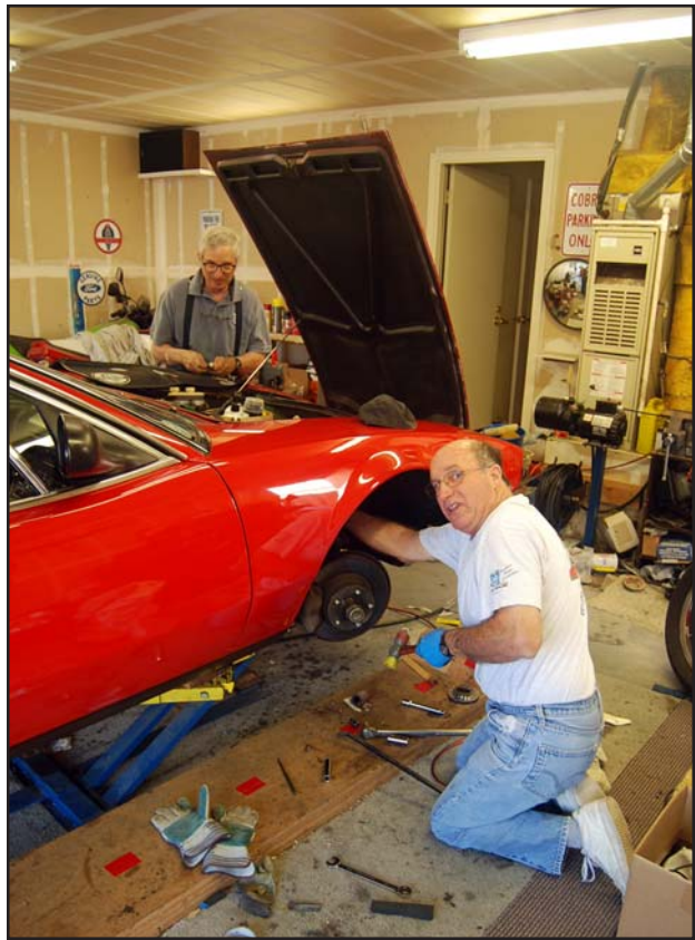
Steve Dalcino removes a front shock while Jim Seiferling (Capitol Panteras co-president) tries in vain to muscle a new headlight limit switch past the radiator
