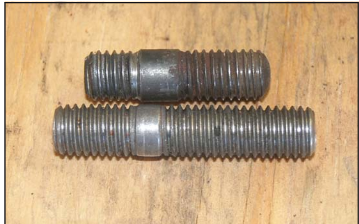
The new starter had a thicker flange, requiring longer starter studs. The holes in the bellhousing had to be tapped further
