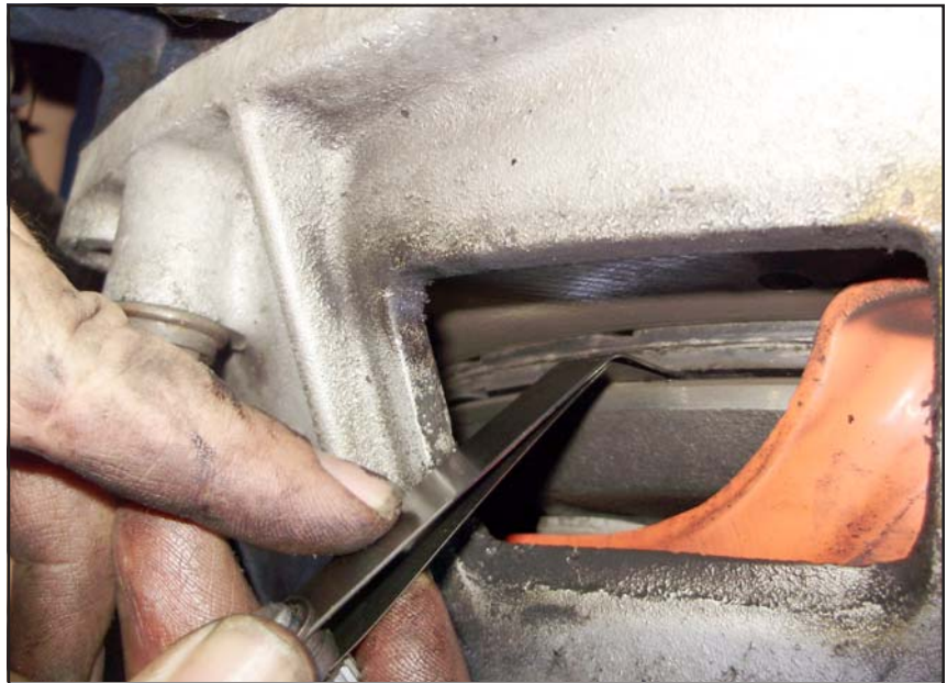
After the clutch was adjusted, a feeler gauge was used to verify the adjustment; the long-throw slave cylinder certainly lived up to its billing, delivering almost twice as much clutch movement as the stock unit
