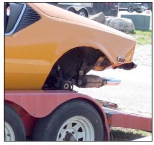
This photo graphically illustrates what happens when axle wear goes undetected and unresolved. Close examination of the photo reveals the wheel bearing, plainly visible, with the snapped-off axle stub still inside.
