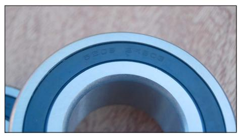
The bearing number is molded into the rubber seal
