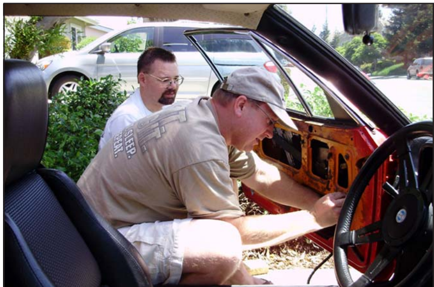
Together, Rich and Brent Stewart changed out Brent's window gears, and got his windows working better than new!
