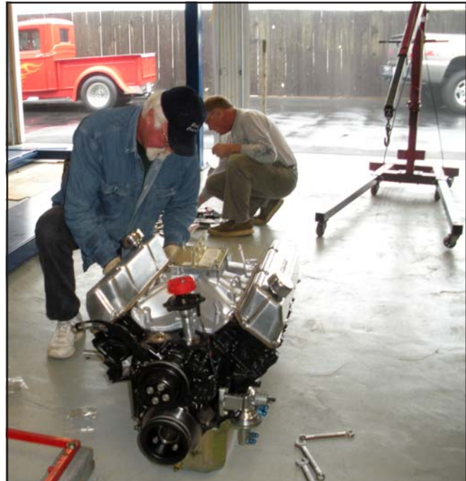
On a dreary, rainy Saturday, Roger Sharp attaches the ZF to the 351C. Note Forest's hot-rod truck in the background
