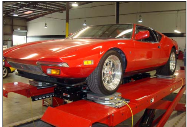
Brent’s Pantera was used to demonstrate the principles of corner-weighting
