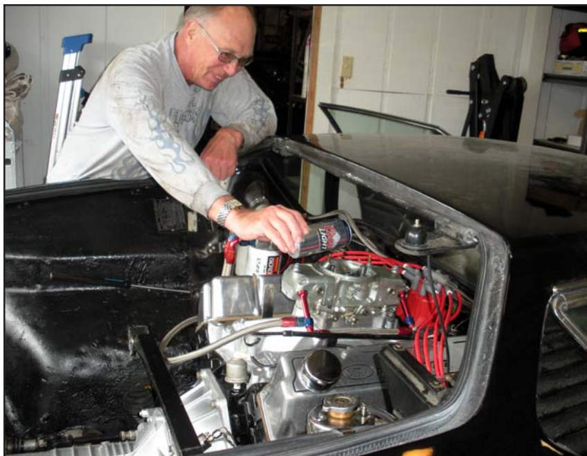
Forest filled an empty beer can (of which there were many to choose from!) with gas, and used it to prime the carburetor for the initial startup
