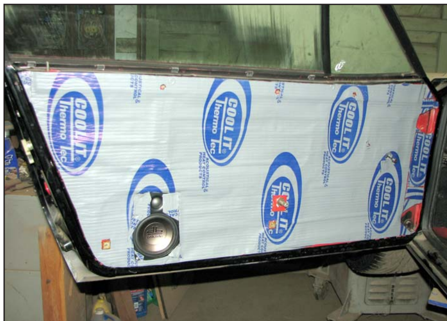
Thermo-Tec Cool-It matting serves as both a noise and heat barrier
