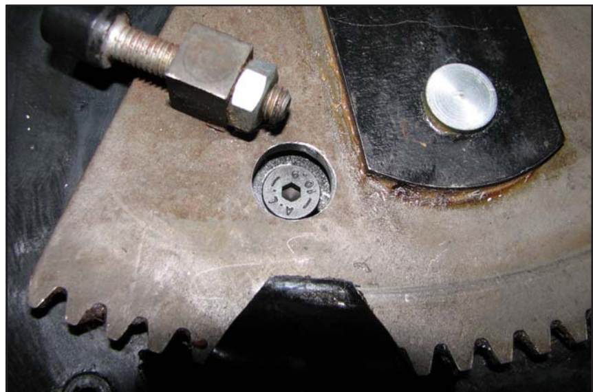
A flat head countersunk socket head cap screw secures the third hole of the motor case; an oversize access hole was created in the gear rack
