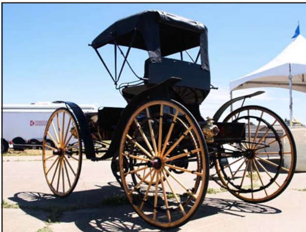
The oldest car present was this 1904 Holsman Hi-Wheeler, which drove into the show under its own power! It uses a two-cylinder engine, with rope drive to the rear wheels
