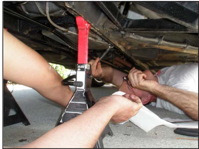
Markus wanted to get his hands dirty, so he got to replace the plastic hydraulic line under the car with a new braided stainless steel line
