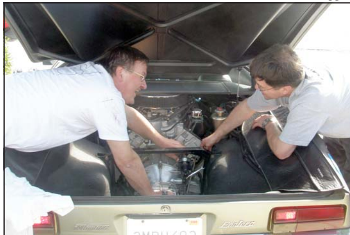
Sebastian Exenberger and Chris Clark worked together to install and adjust the slave cylinder
