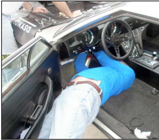
Lee Farrell demonstrates that it is much easier to remove the master cylinder with two people; one holds the nuts while the other turns the bolts
